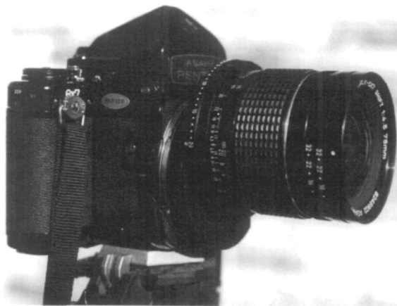
A medium-format camera mounted on a tripod with a 75-mm shift lens. (Jeff Dean, 1980)
