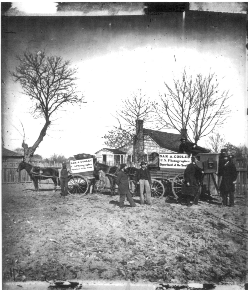
Taken near Savannah, Georgia this photograph shows a typical field set-up of the Civil War era. The wagon carried chemicals, glass plates, and negatives. The buggy to the left could be used as a field darkroom. Before a reliable, dry-plate process was invented (ca. 1879) photographers had to develop negatives quickly before the emulsion dried. (Library of Congress, Prints and Photographs Division)
