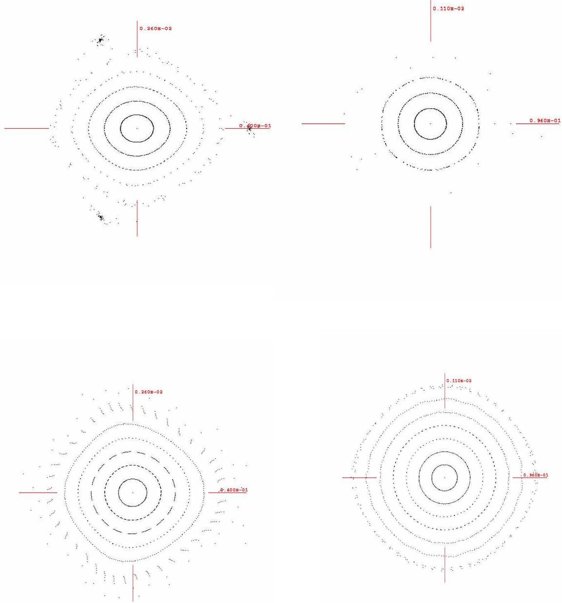
**Figure 11:** Top: Horizontal (left) and vertical (right) accepted phase space plots obtained by 9<sup>th</sup> order tracking through the full muon storage ring, including chromatic correction sextupoles and quadrupole fringe fields. Tracking is plotted in steps of  $0.5 \sigma$  for an normalized emittance (rms) of  $3200 \pi$  mm-mr. Bottom: Same as top plots but with quadrupole fringe fields in the matching sections to the production straight turned off.
