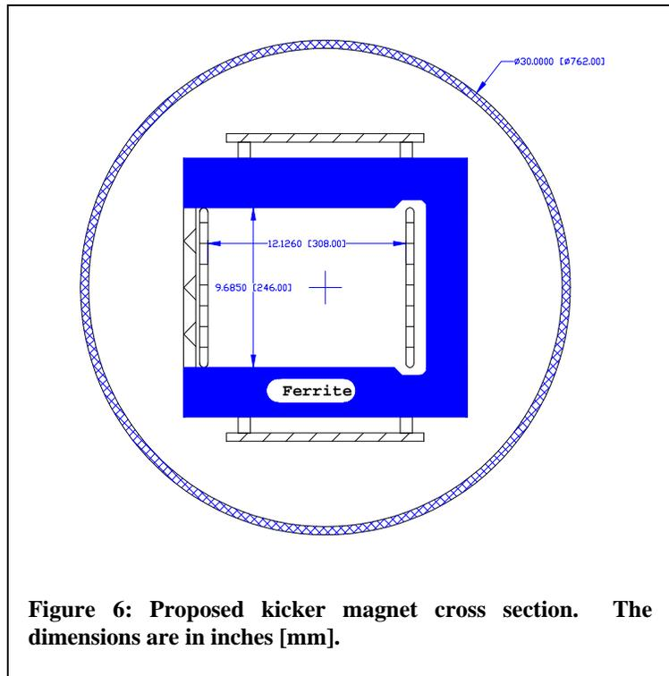
**Figure 6:** Proposed kicker magnet cross section. The dimensions are in inches [mm].
