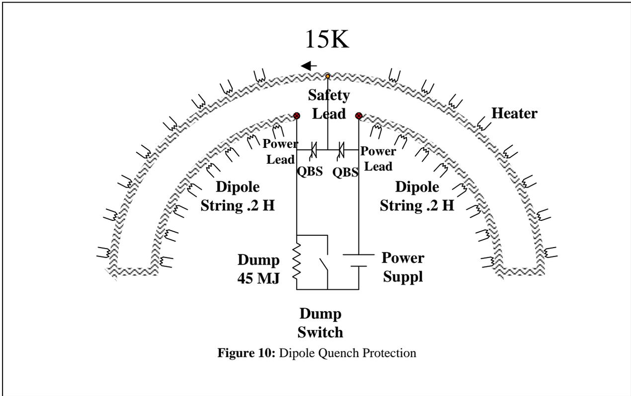
Figure 10: Dipole Quench Protection
