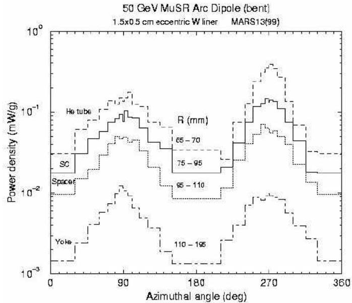
**Figure 13:** Power density in the bent arc dipole.
