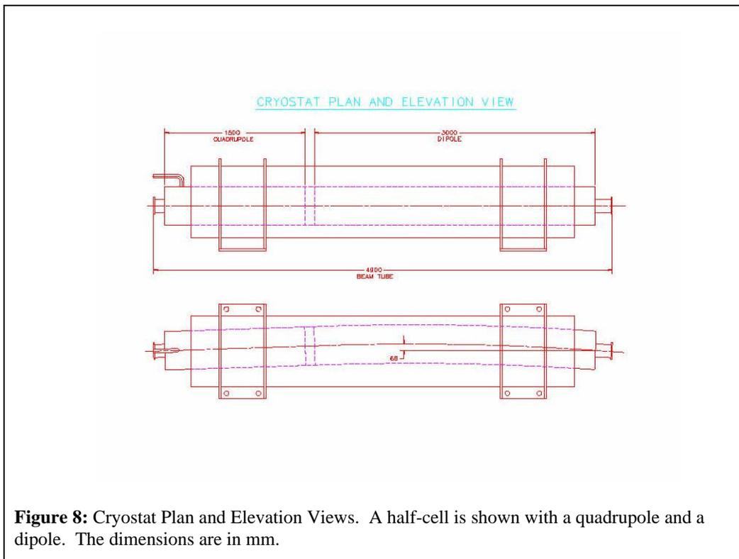
**Figure 8:** Cryostat Plan and Elevation Views. A half-cell is shown with a quadrupole and a dipole. The dimensions are in mm.
