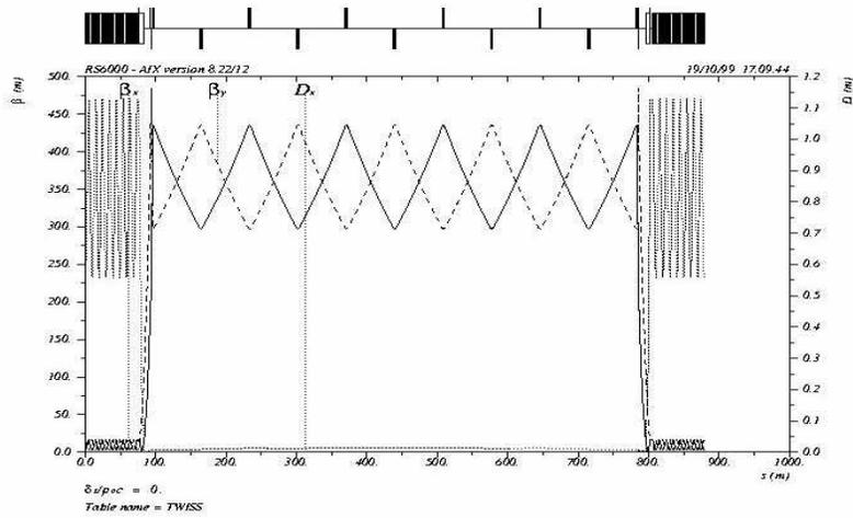
Figure 4: Lattice functions in the production straight.
