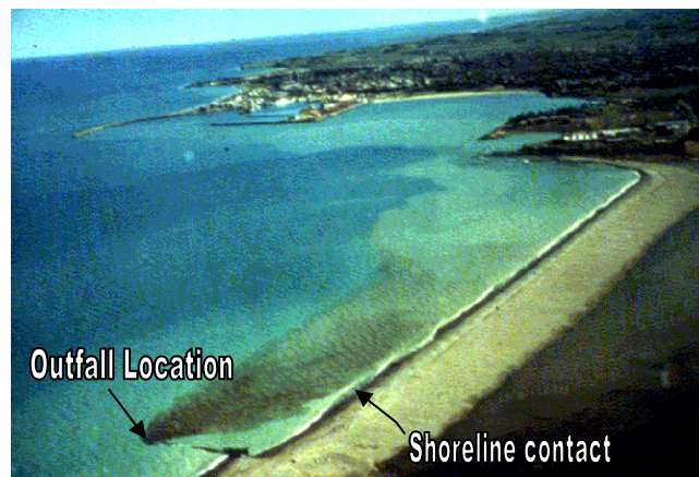
Figure 1. Example of a wastewater outfall and shoreline plume boundary interaction. The wastewater plume contacts the shoreline and exhibits upstream density current buoyant spreading. Due to the shallow water discharge location, near-field instabilities with significant benthic and shoreline impacts are likely. (Photo by I. Wood).
