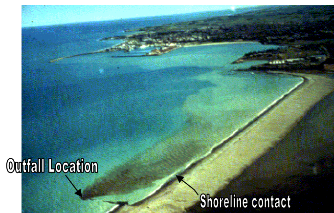
Figure 1. Example of a wastewater outfall and shoreline plume boundary interaction. The wastewater plume contacts the shoreline and exhibits upstream density current buoyant spreading. Due to the shallow water discharge location, near-field instabilities with significant benthic and shoreline impacts are likely (Photo: I. Wood).
