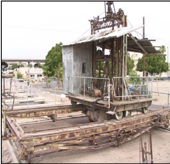
Figure 3.—Blaisdell slowsand filter washing machine in Yuma, Arizona (photo by Paul McAleese, June 2002).
