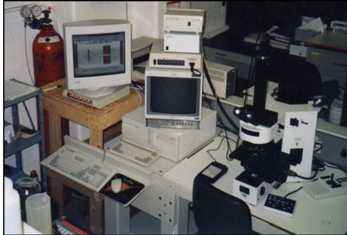
Figure 1-6 – Olympus AX 70 Microscope, Optronics CCD Camera, and Sony Monitor.
