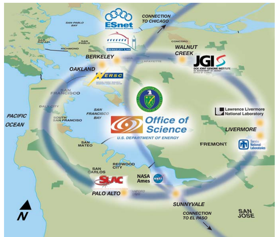
FIGURE 11. ESnet's new San Francisco Bay Area Metropolitan Area Network provides dual connectivity at 20 to 30 gigabits per second to six DOE sites and NASA Ames Research Center.
