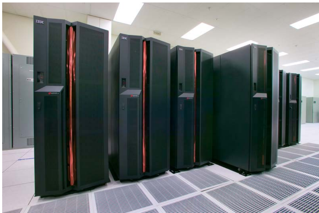
FIGURE 8. Bassi is an 888-processor IBM p575 POWER5 system with a theoretical peak performance of 6.7 teraflop/s.
