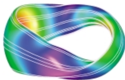
Quasi-Poloidal Stellarator (QPS) optimized stellarator plasma surface with magnetic field line (white) superimposed.
