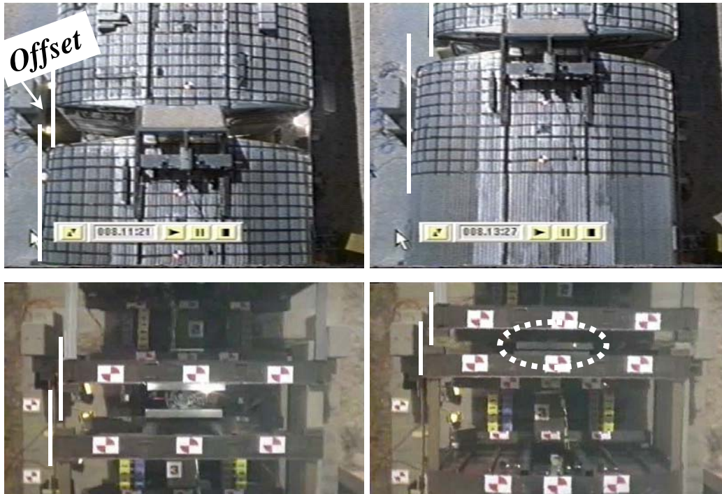
Figure 30. Still photographs of the coupled interface in the conventional (top) and CEM (bottom) tests at time of impact (left) and maximum crush (right)
