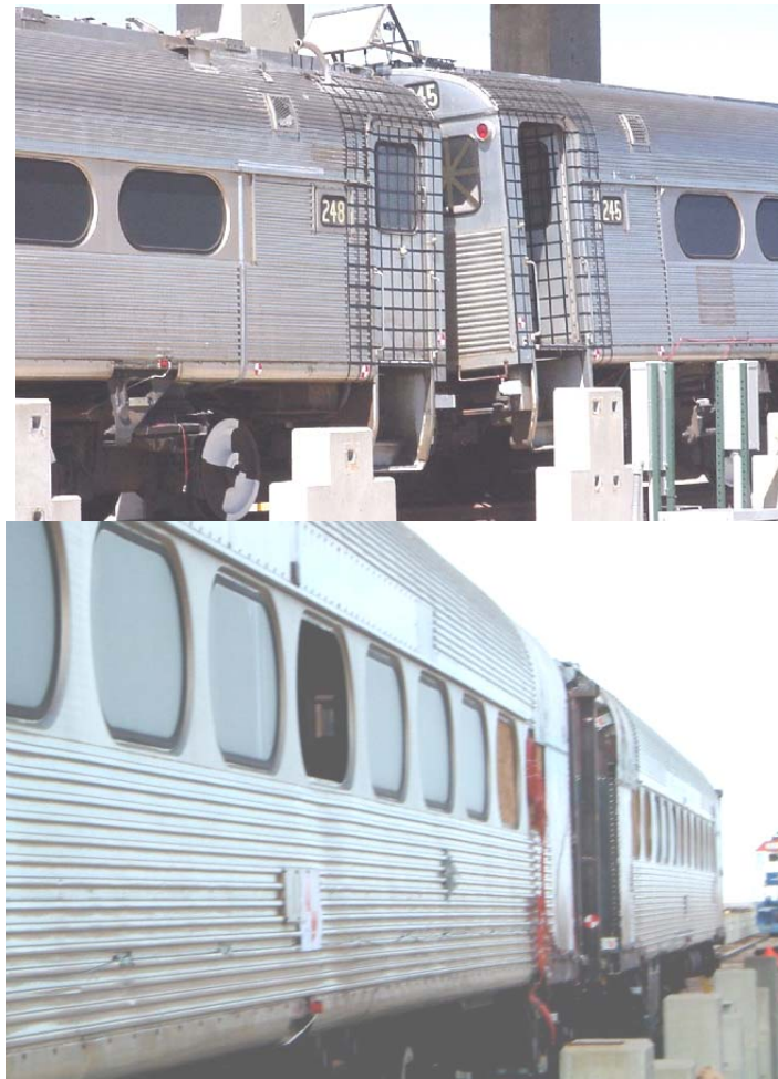
Figure 29. Post-test photographs from the two-car test of the conventional (top) and CEM (bottom) coupled connections
