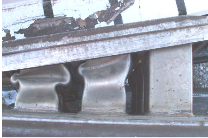
Figure 38. Post-test photograph of the deformable anti-climber, showing no material failure
