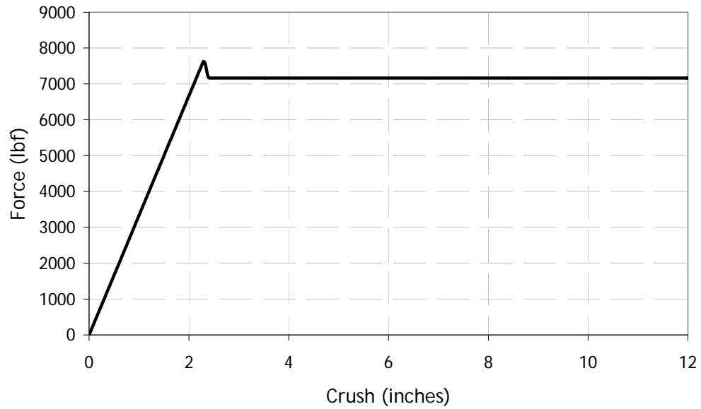
Figure 73. Single-car model exercised with lateral perturbation: results of the derailment characteristic, force vs. displacement between the truck and dummy mass
