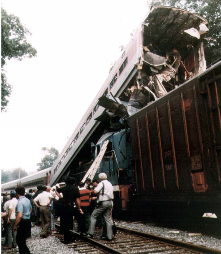
Figure 4. Train-to-train accident with override; Beverly, Massachusetts - August 11, 1981
