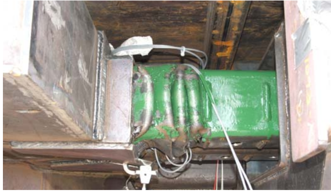
Figure 37. Post-test photograph of a primary energy absorber, showing material failure along the bottom folds of the crushing cells
