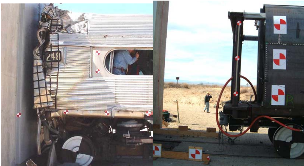
Figure 28. Post-test photographs from the two-car impact test of the lead conventional (left) and CEM (right) vehicles
