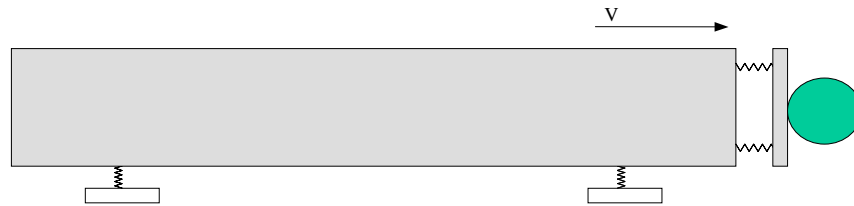
Figure A-26. Schematic of Lumped-Mass CD Model
