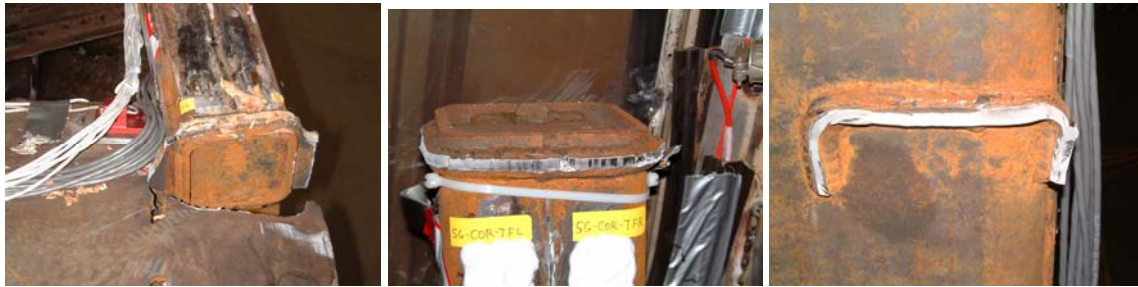
Figure A-24. Post-Test Photographs of Material Failure in 1990s Design, Corner Post Connection to End Beam, Failed Connection at Top of Corner Post, and Failed Connection to Shelf on Collision Post
