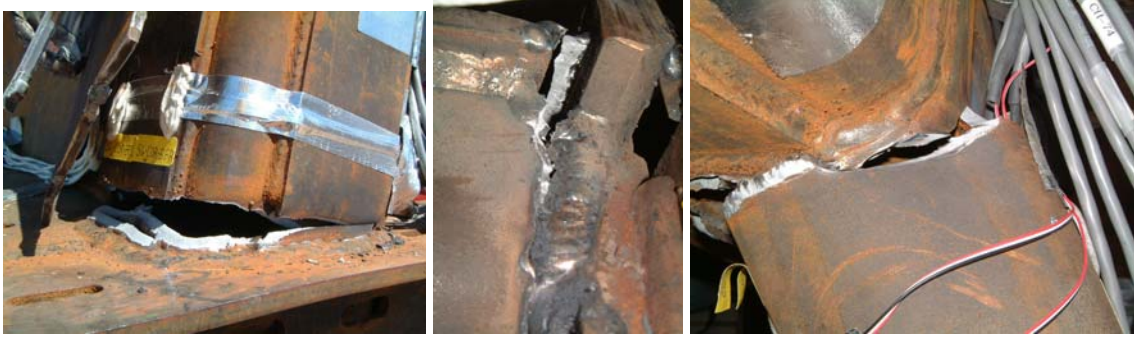
Figure A-25. Post-Test Photographs of Material Failure in SOA Design, Corner Post Connection to End Beam, AT Plate Connection to Roof Plate, and Shelf Connection to Collision Post
