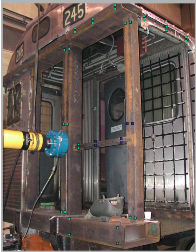
Figure B-7. Strain Gauges on 1990s End Frame Design
