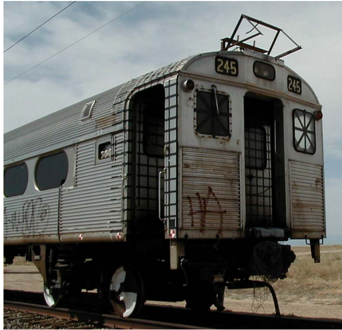
Figure 6. One of the Budd Pioneer Cars Prior to Modification for this Program. (The Stairwell has been Removed)
