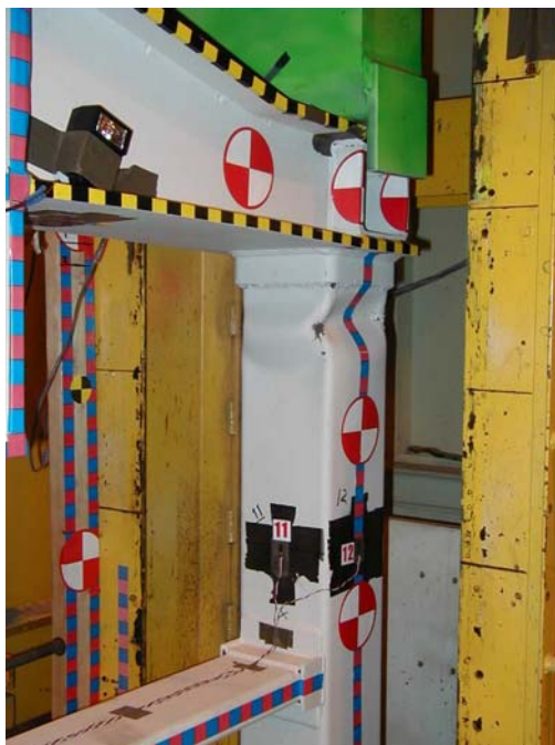
Figure 3. Full-Scale End Beam/Side Sill Corner Post Support Element Designed and Tested to Demonstrate Substantial Energy Absorption Capability
