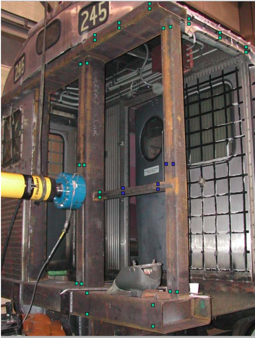
Figure 26. End Frame Quasi-static Loading Test Arrangement; Strain Gage Locations are Shown by the Small Colored Points
