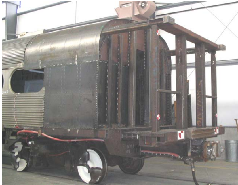
Figure 2. Crush Zone End 244B Before Testing
