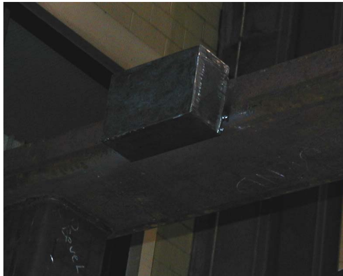
Figure 20. Newly Added Center Spacer on the AT Beam to Reduce Its Bowing When Coupled Ends Collide
