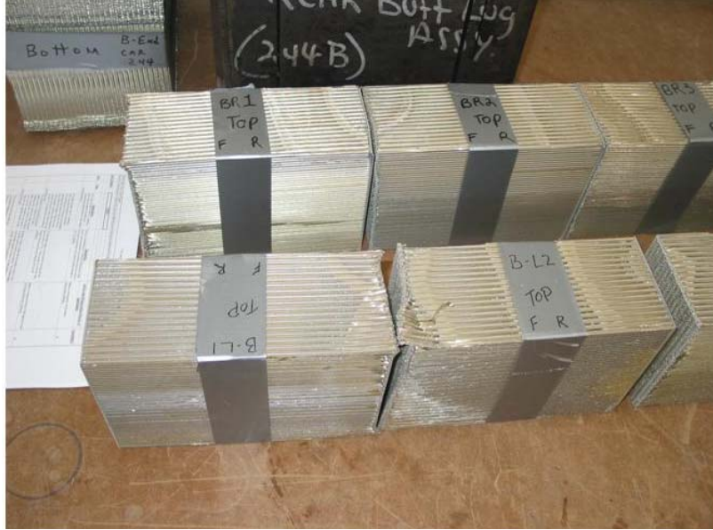
Figure 14. Aluminum Honeycomb Roof Absorber Elements from End 244B After the Two-Car CEM Test
