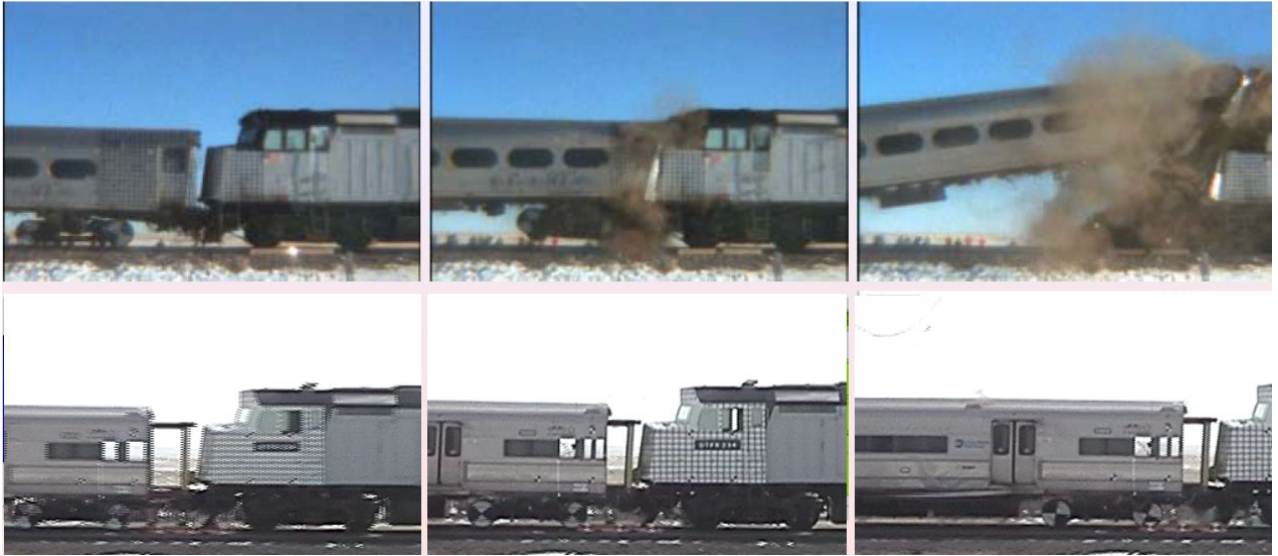
Figure 5. Frames from Train-to-Train Test Movies of CEM and Existing Equipment
