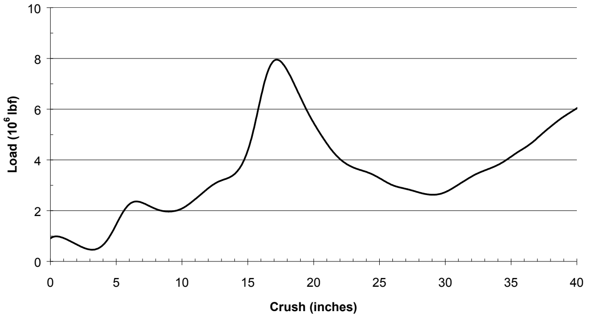
Figure 45 - The Load-Crush Response for the Combined Locomotive Anticlimber/End Underframe Crush Zone.
