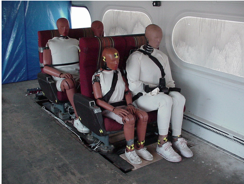
Figure 3. Inter-city passenger seat incorporating lap and shoulder belts.
