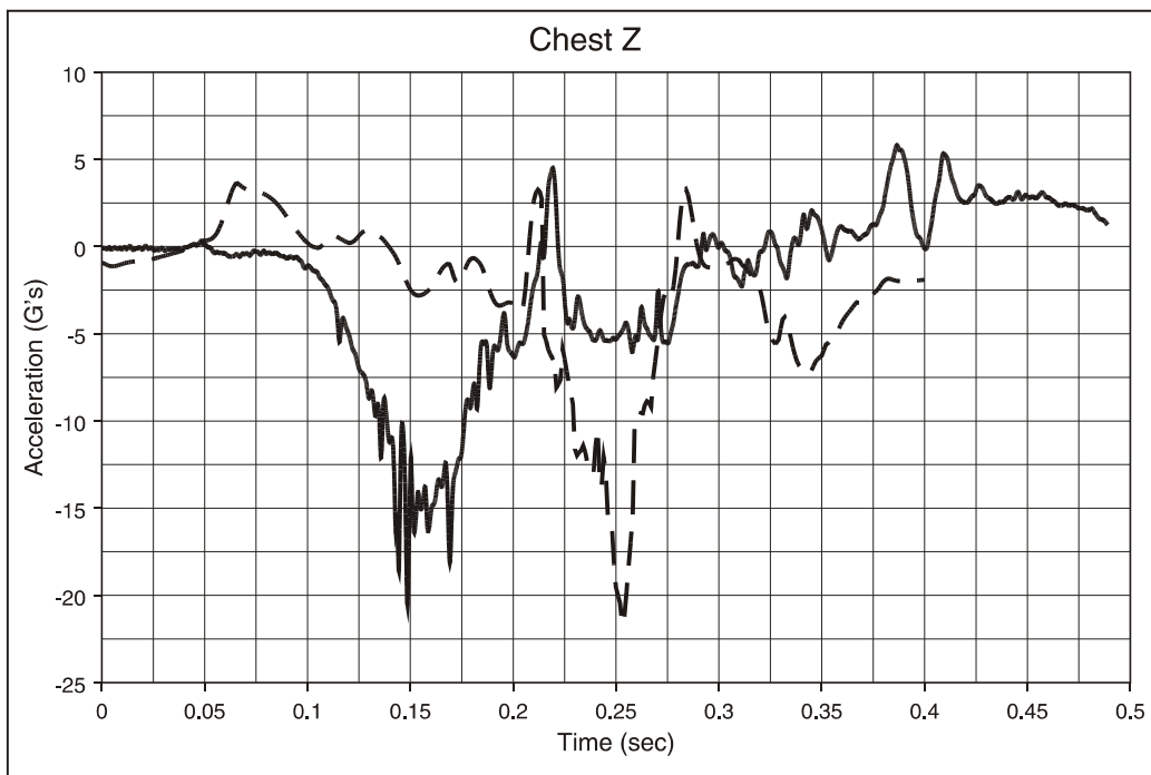
Figure F144. Walkover Seat, Type 1 Test, 50th-Percentile Hybrid II Male ATD, Aisle Seat; Chest Acceleration, z Direction
