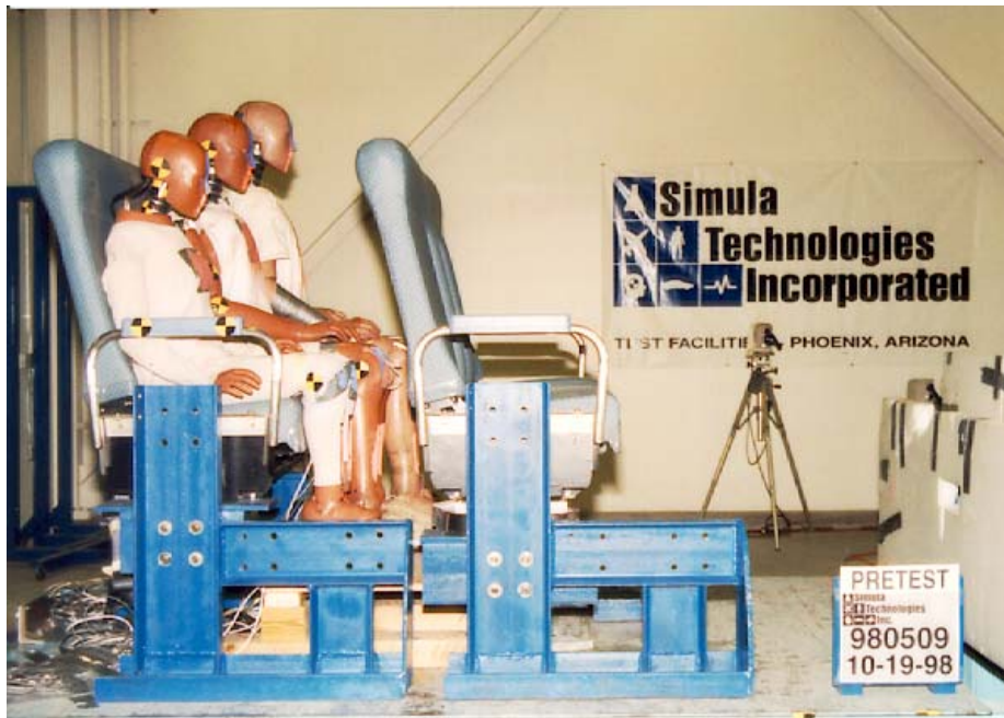
Figure 22. Type 2 Test - 95th-Percentile Male, 50th-Percentile Male, and 5th-Percentile Female ATDs -Hybrid III 5th-Percentile Female in Window Seat, Hybrid III 50th-Percentile Male in Middle Seat, and Hybrid III Male 95th-Percentile in Aisle Seat
