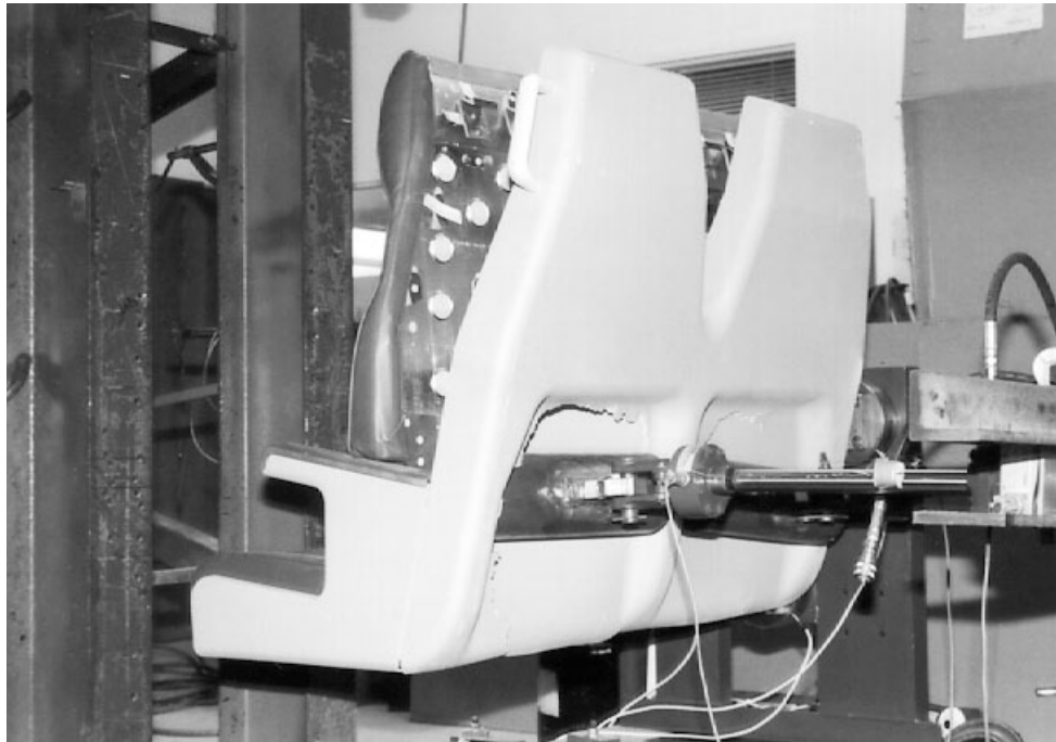
Figure 13. C-3 Lower (Post-test) - Plastic Shroud Cracked and Back Cushions Detached
