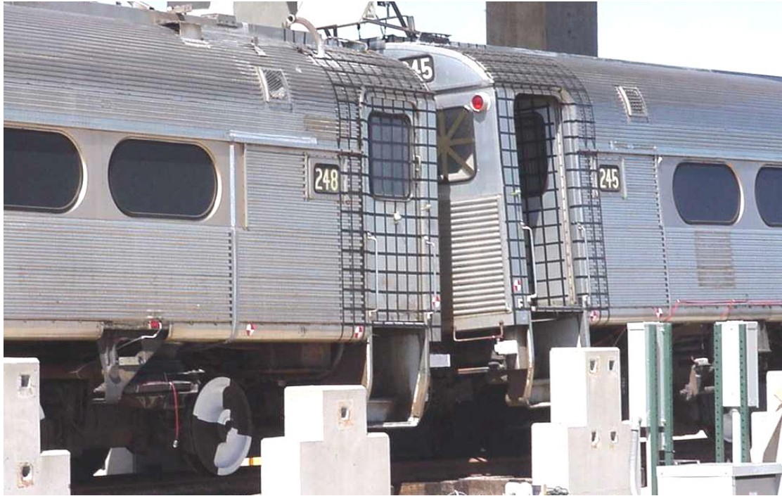
Figure 20. Photo of Coupled Connection After Two-Car Impact Test
