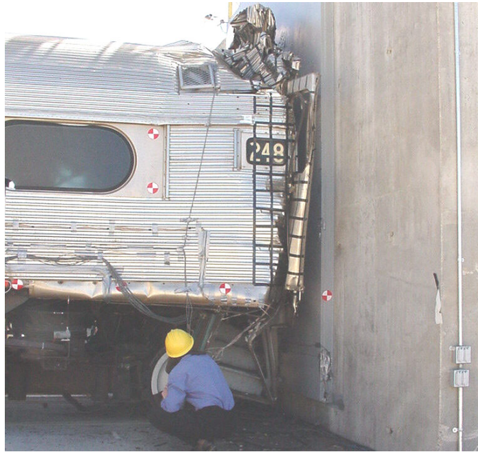
Figure 17. Photo of Impact End of Leading Car After Two-Car Impact Test
