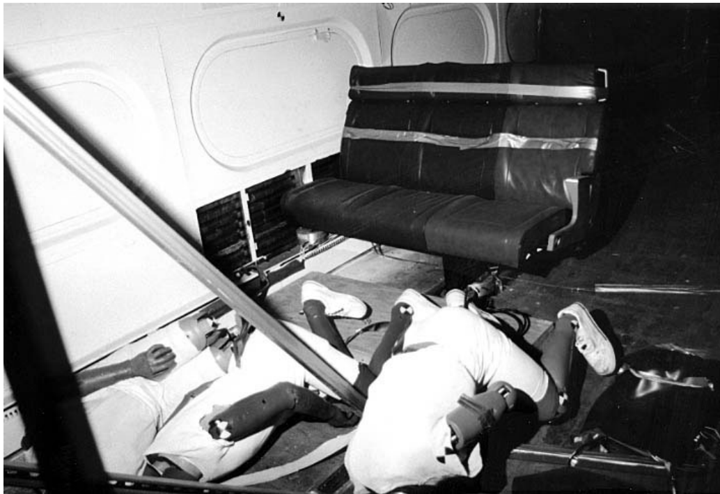
Figure 12. Experiment No. 1-3 – Post-Test Photograph of ATDs on the Floor Following Rebound
