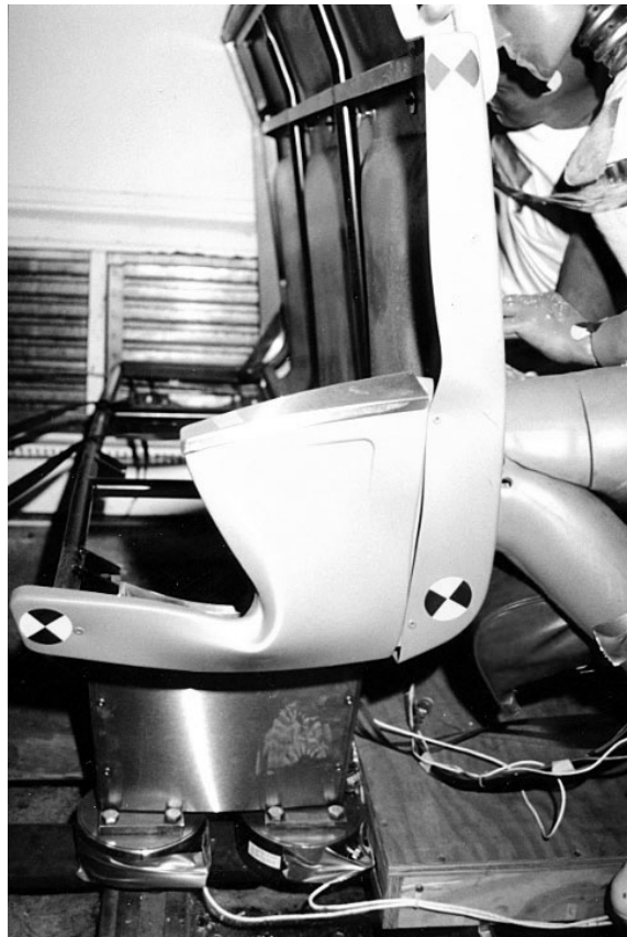
Figure 3. Experiment No. 1-1 – Post-Test Seat Photograph of Pedestal and Side Arm Shroud Deformation
