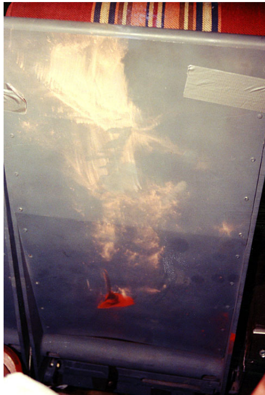
Figure 9. Experiment No. 1-2 – Post-Test Photograph of Seat Back Deformation Due to Knees Impacting from Behind
