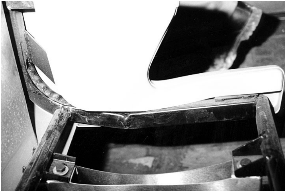
Figure 5. Experiment No. 1-1 – Post-Test Photograph of Side Arm Frame and Shroud Deformation
