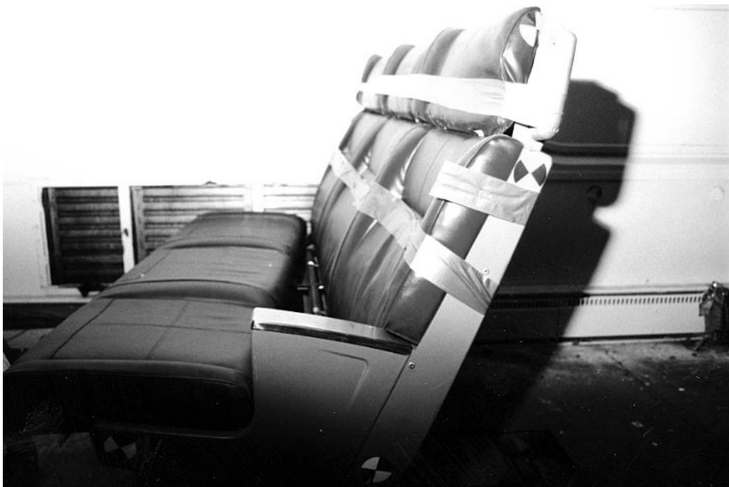
Figure 11. Experiment No. 1-3 – Post-Test Photograph of Seat Back Deformation
