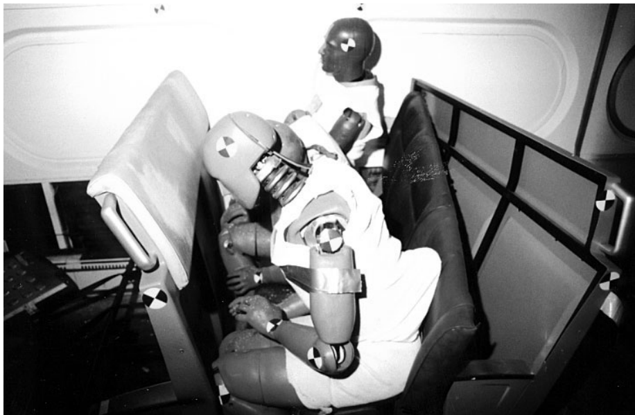
Figure 4. Experiment No. 1-1 – Post-Test Photograph where Occupants Remain Compartmentalized
