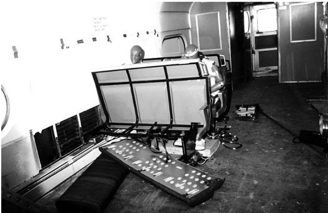
Figure 6. Experiment No. 2-1 – Post-Test Photograph where Seat Occupants Remain Compartmentalized
