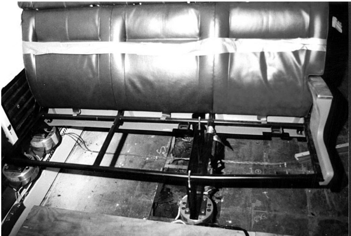
Figure 10. Experiment No. 1-3 – Post-Test Photograph of Seat Frame Deformation
