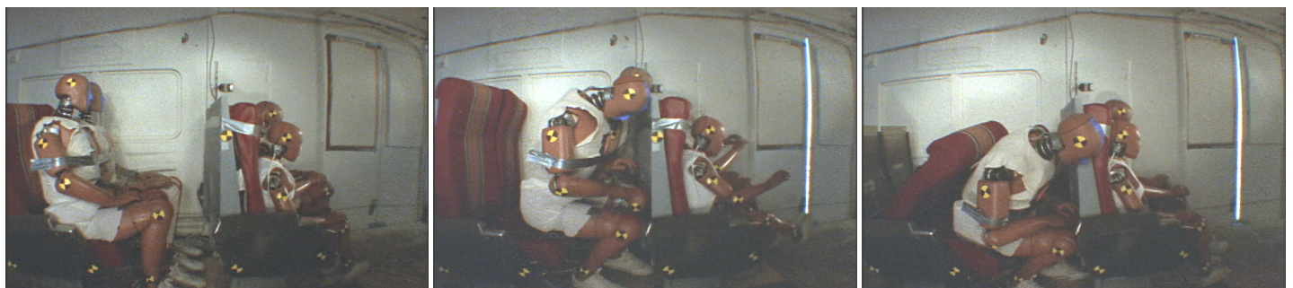
Figure 17. Time-Sequence for Experiment 2-1, Forward-Facing Inter-city Seats with and without Restraints
