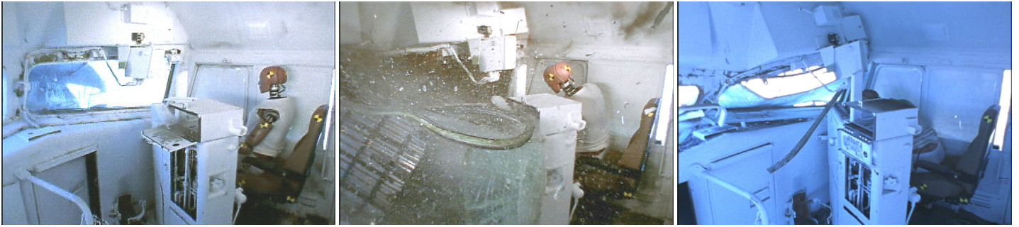
Figure 10. Time-Sequence for Experiment L-1, Locomotive Operator's Seat
