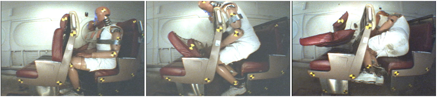
Figure 13. Time-Sequence for Experiment 1-1, Forward-Facing Commuter Rail Passenger Seats in Cab Car
