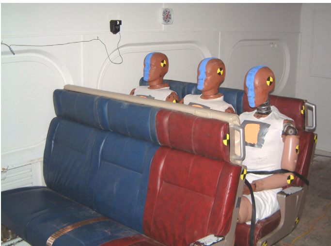
Figure 11. Pre-test photo of Experiment No. 1-1, Forward-Facing Commuter Rail Passenger Seats in Cab Car
