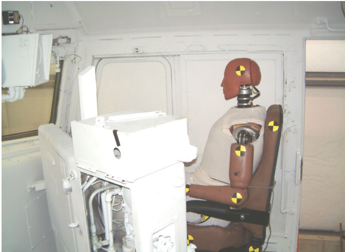
Figure 8. Pre-test photo of Experiment No. L-1, locomotive operator seat
