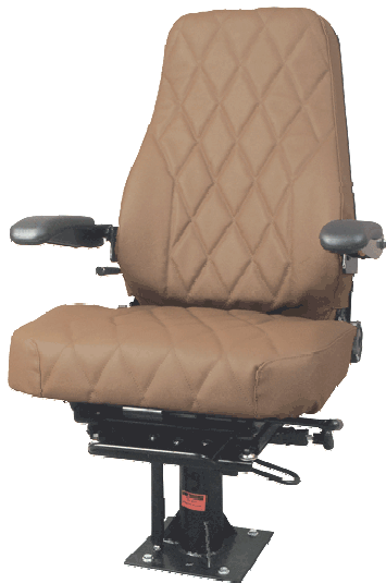
Figure 9. Locomotive operator, high-back seat, manufactured by Seats, Inc.
