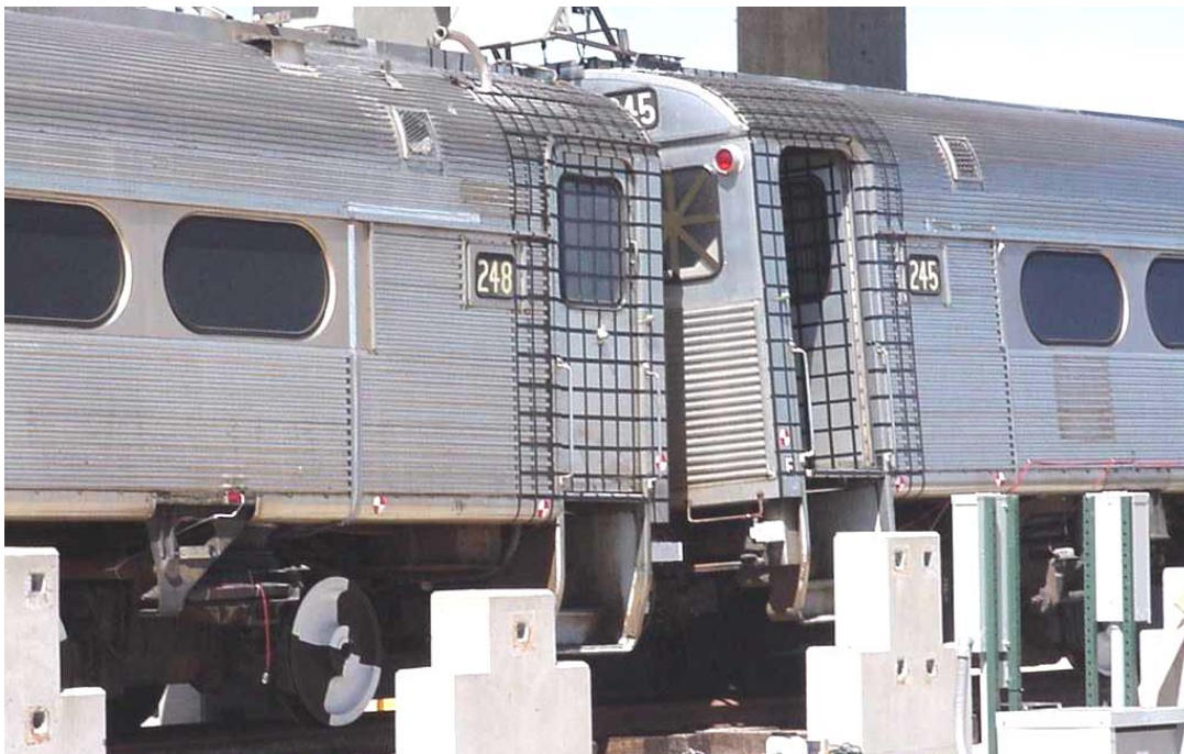
Figure 10. Photograph of coupled connection after two-car test.
