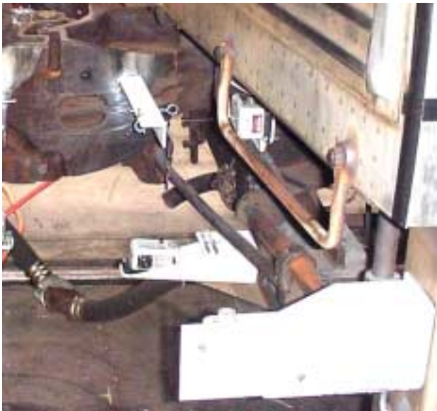
Figure 22. Photograph of Displacement Transducers on Coupler of Trailing Car
