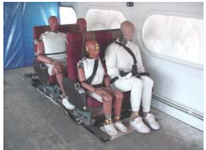
Figure 11. Amtrak Traditional Coach Seats, Leading Seat Modified with Lap and Shoulder Belts
