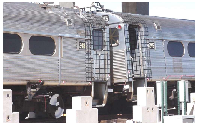
Figure 12. Photo of Coupled Connection After Two-Car Test
