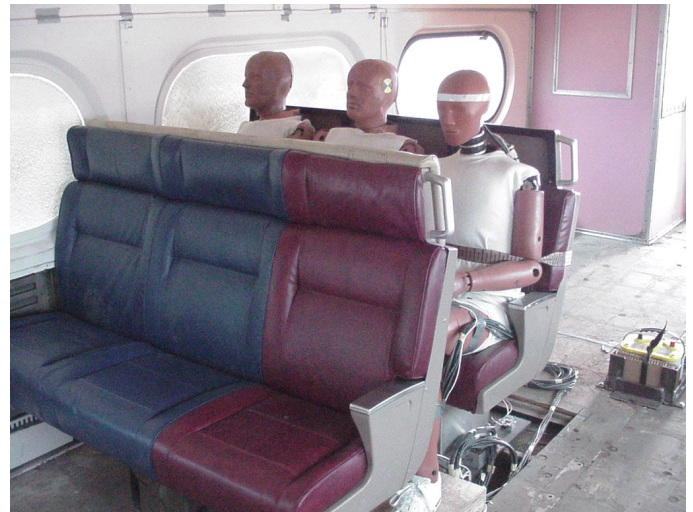
Figure 9. Experiment 2-1, Forward Facing Rows of Seats, Trailing Car, Pre-Test
