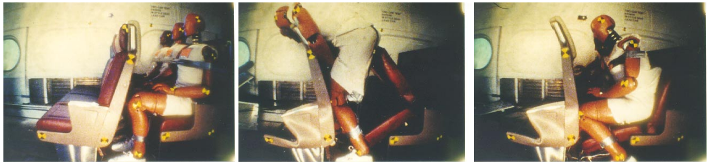
Figure 14. Time-Sequence for Experiment 1-1, Forward Facing Rows of Seats, Leading Car
