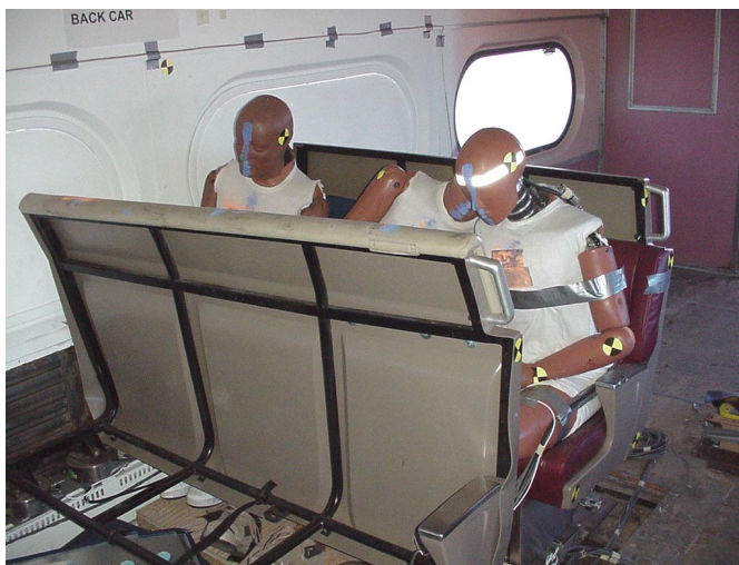
Figure 12. Experiment 2-1, Forward Facing Rows of Seats, Trailing Car, Post-Test
