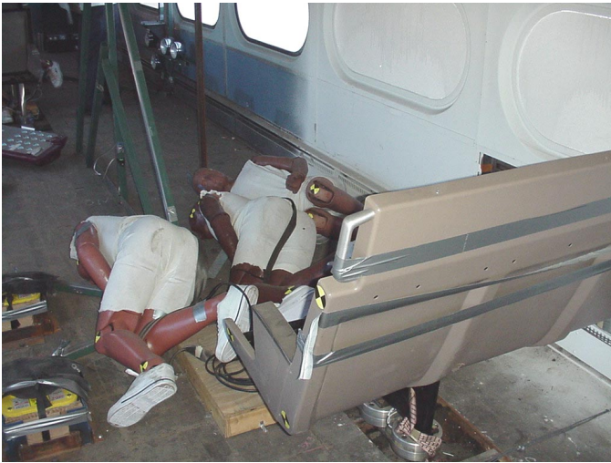
Figure 21. Experiment 1-3, Rear Facing Rows of Seats, Leading Car, Post-Test
