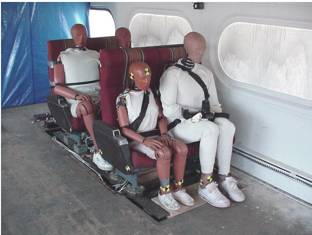
Figure 16. Experiment 1-2, Forward Facing Rows of Seats with Lap and Shoulder Belts, Leading Car, Pre-Test
