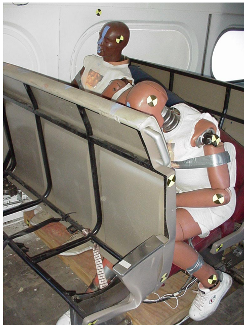
Figure 15. Experiment 1-1, Forward Facing Rows of Seats, Leading Car, Post-Test
