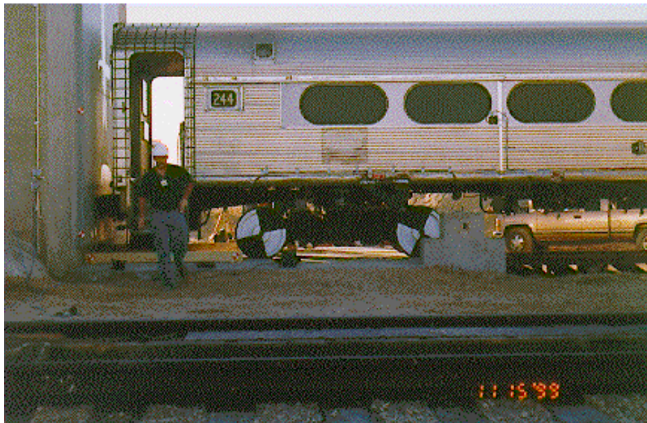
Figure 5-2. Photo of Impact End of Car Prior to Single-Car Test
