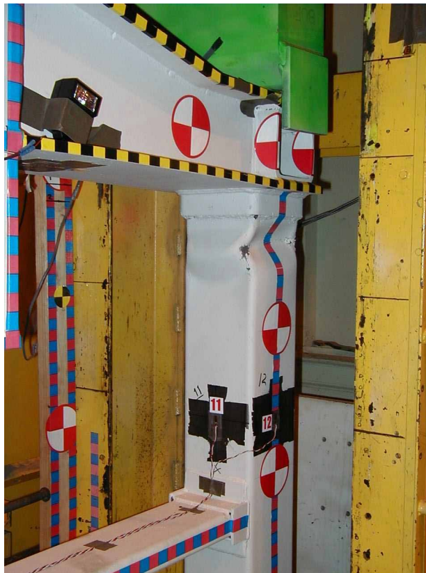
Figure 13: Photograph of the Modified End Beam at the Top of the 'Side Sill' Element after the First Impact
