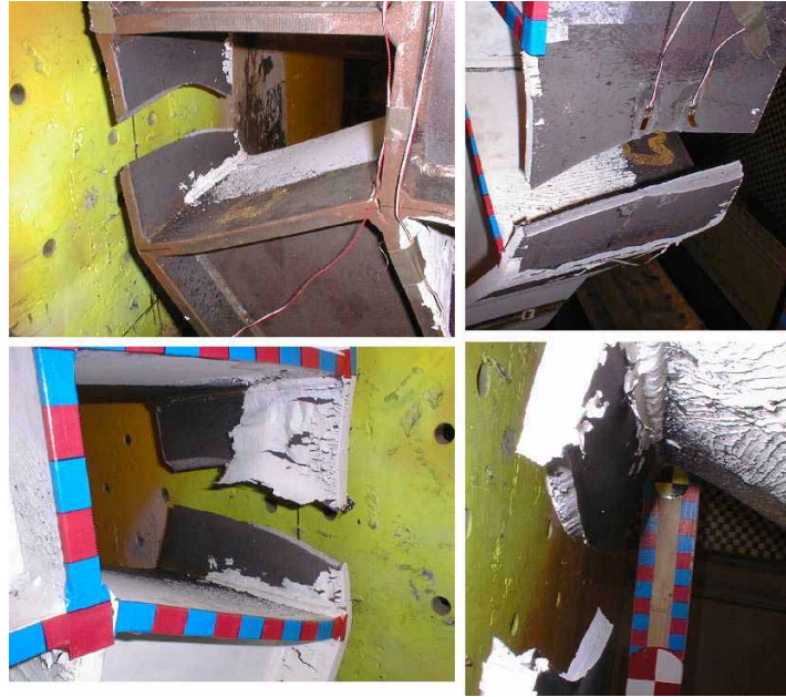
Figure 11: Close-Up Photographs of the Fracture Location in the Quasistatic, Baseline End Beam Test
