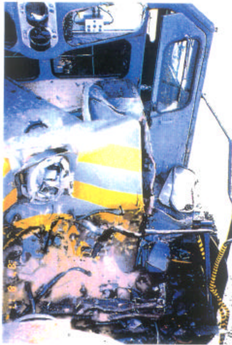
Figure 4-11. Front View Photograph of the Overridden Lead Locomotive in Scenario C, Showing the Limited Short Hood Structure Crush
