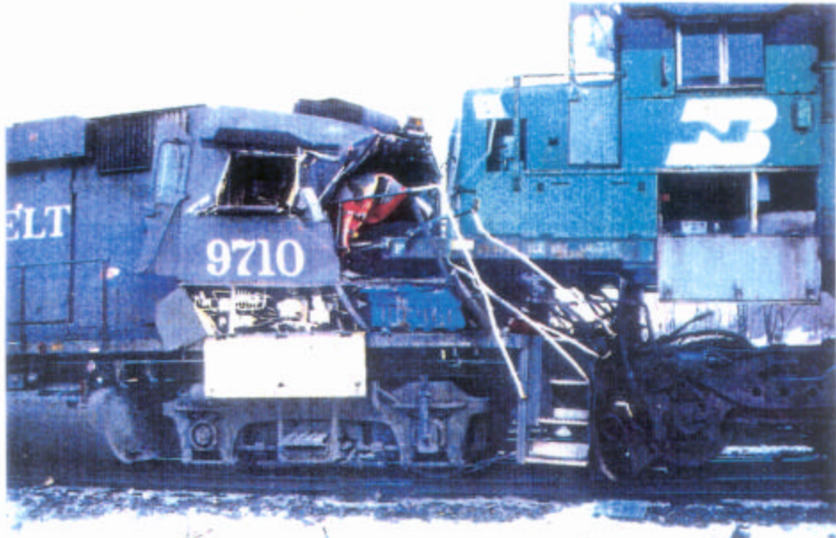
Figure 4-6. Photograph of the Override between the Two Lead Locomotives in Scenario B, 30 mph Closing Speed
