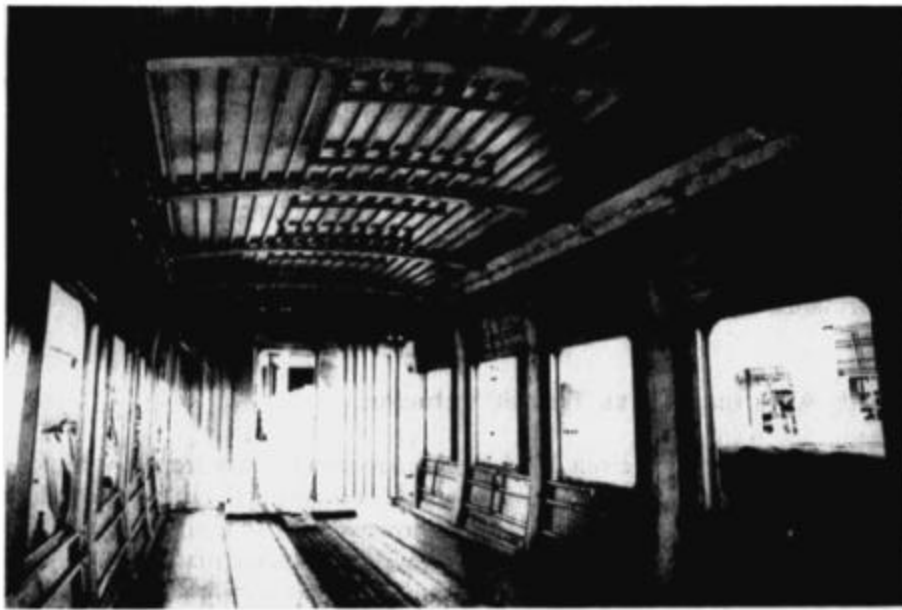
Figure 5-4 Typical Talgo HSGGT Passenger Coach Superstructure
