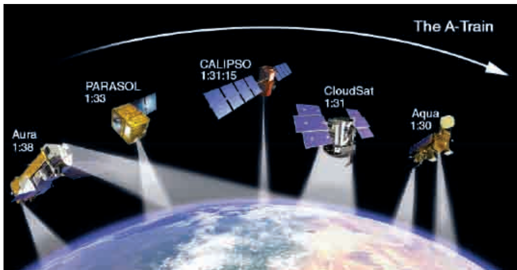
Figure 2.5. A constellation of five spacecraft that overfly the Equator at about 1:30 PM, the so-called A-Train, carries sensors having complementary capabilities, offering unprecedented opportunities to study aerosols from space in multiple dimensions.
