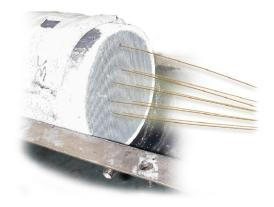
Minimally invasive SPACI-MS (spatially resolved capillary inlet mass spectrometry) uses capillary tubes to sample emissions inside catalyst monolith channels, engine intake ports, and so forth.
