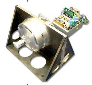
In a collaborative effort between ORNL and Rockwell Scientific, an all-silicon carbide power module is being developed and built. Silicon carbide meets the performance requirements for future transportation applications, but research and development is needed to resolve issues related to cost and processing.
