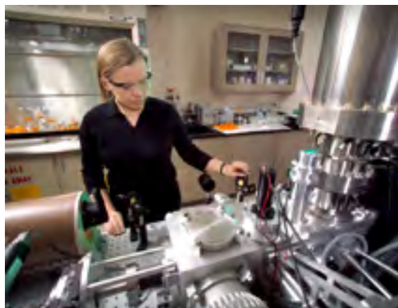
Figure 12. EMSL’s field-deployable second-generation single particle laser ablation time-of-flight mass spectrometer—or SPLAT II—is a high-precision and unique instrument that allows researchers to study the fundamental processes that govern the chemistry and physics of aerosol particles on the nano- and micro-scales.
