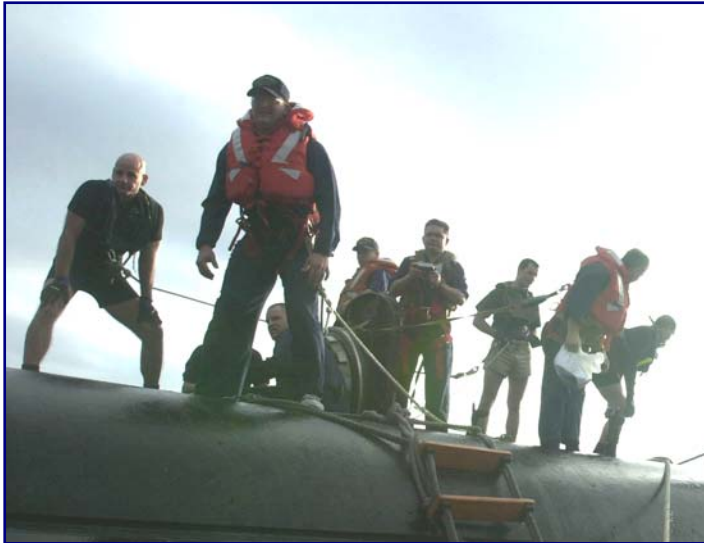
Crewmembers wearing fall protection on USS Greenville (SSN 772).
