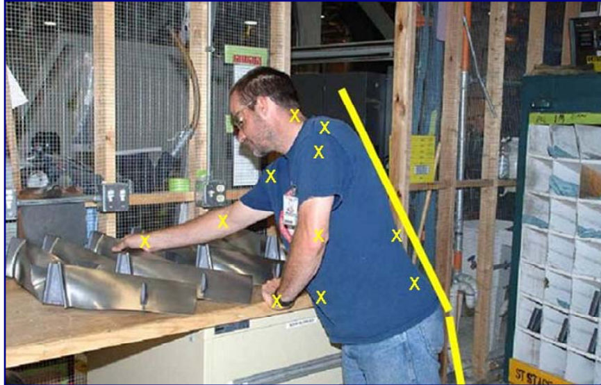
Work at Mass Moment Stations used to involve standing for long periods and awkward reaches.
