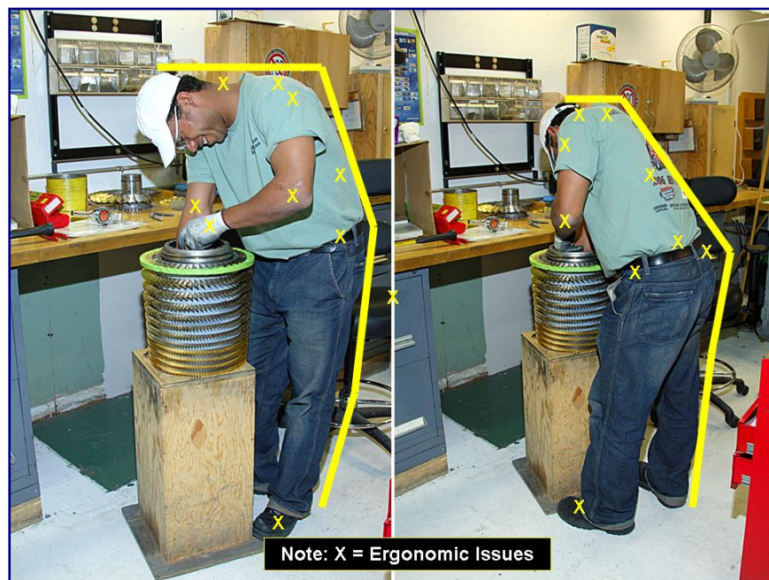
Artisans stood for long periods bent over T64 compressors, putting them at risk for WMSDs.
