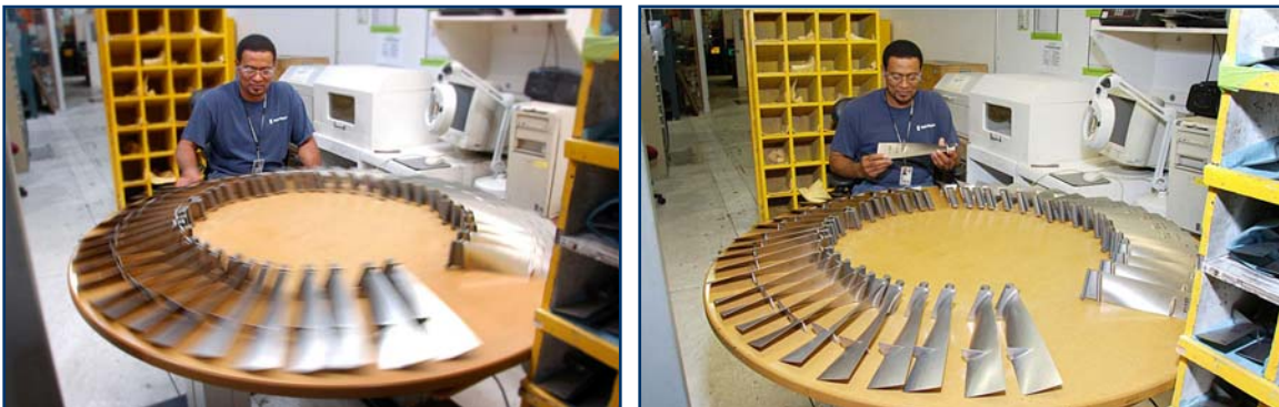
At Mass Moment Stations, the Lazy Susan can be adjusted to allow artisans to alternate sitting and standing postures and rotates to eliminate the need for awkward reaches.
