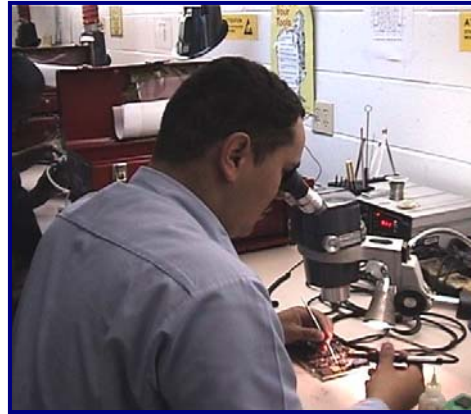
Technician uses microscope to aid in soldering small electronics part.
