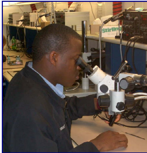
Adjustable microscopes allow technicians to work in neutral positions.
