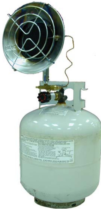
Figure 8. Photograph of sample tank-top heater used in tests
