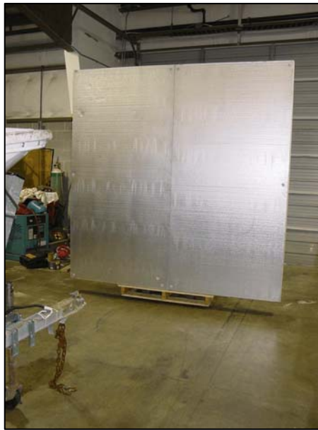
Figure 3. Air gap sensor test target
