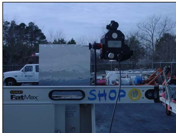
Figure 6. Laser range finder affixed to air gap sensor mounting bracket
