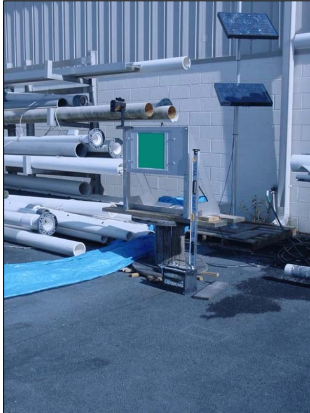
Figure 4. Air gap sensor mounting bracket
