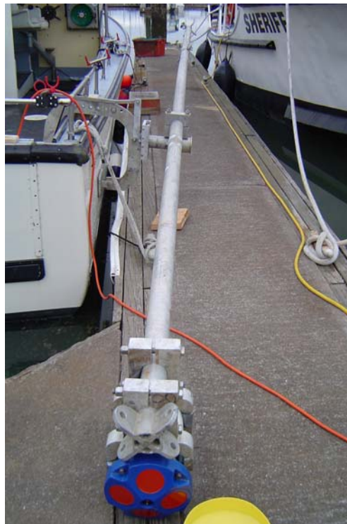
Pole Mounted Towed ADCP mount
