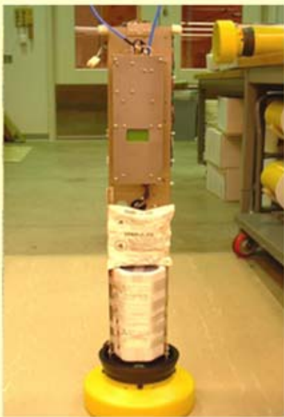
Drifter with Iridium unit installed.
