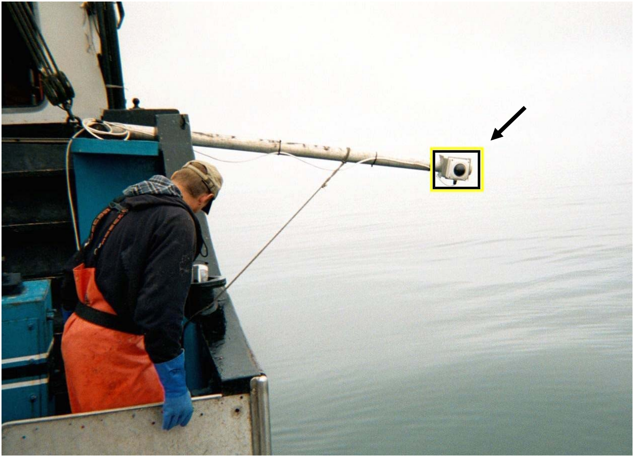
Figure 9. Mounting location and relative position of the roller camera on the F/V Heritage .
