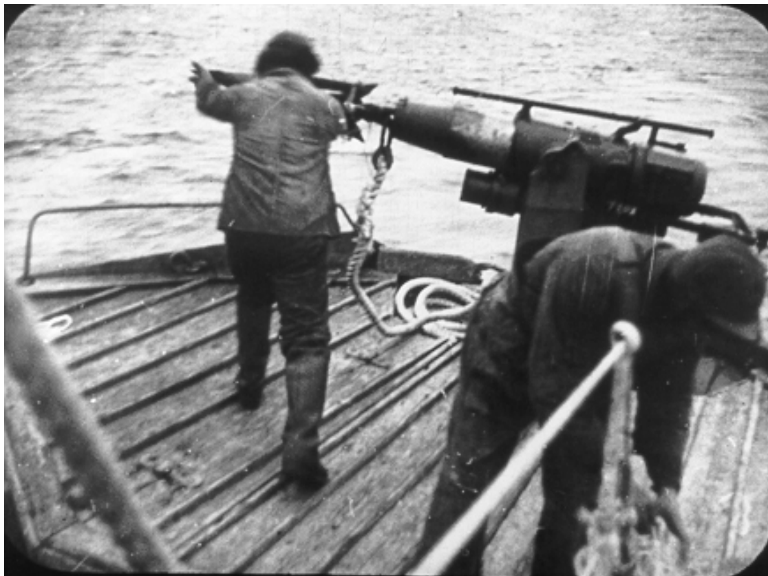
Fig. 7. "Eight killer boats and one factory ship constitute the whaling fleet. Each killer boat mounts a gun like this one, ready to shoot a harpoon into the target." "This 3.5" cannon fires a harpoon six feet in length and weighing between 100 and 200 pounds. The harpoon is pointed with a hollow cast iron bomb which is filled with black blasting powder. This bomb is exploded in the whale's vitals by a time fuse that ignites the powder three seconds after the harpoon has left the gun. The harpoon line coiled on the pan [at the bow] is connected to 1,000 or more fathoms of heavier manila hawser in the forward hold."
