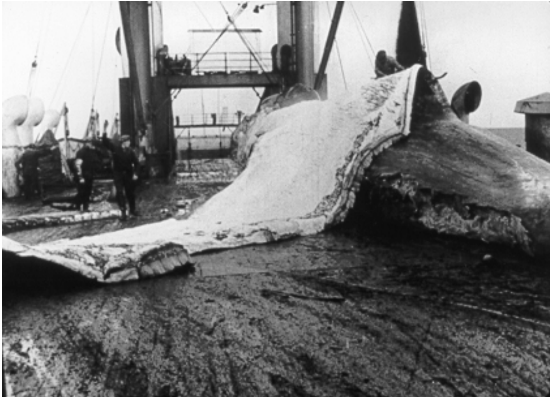
Fig. 16. "The two free strips of blubber are simultaneously peeled off by wires from steam winches."
