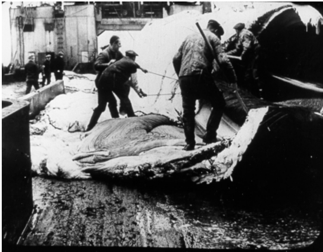
Fig. 19. “The blubber is drawn away to the sides of the flensing deck where it is cut into smaller pieces and then dumped into the cookers or blubber boilers which line both sides of the deck. A number of steam jets open into the cookers, and these rapidly melt out the oil.”
