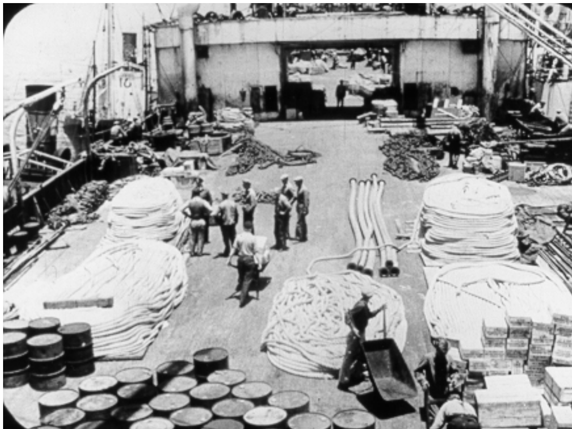
Fig. 3. The deck of the Ulysses . “The Ulysses [was] one of the two floating factories registered under the American flag, the other being the Frango . The Ulysses [was] a 12,395 ton vessel and is 514 feet in length. The Frango [was] 6,400 tons, length 401 feet. Floating factories [were] in operation [in the 1930s] of over 30,000 tons. These vessels with their fleet of six or more fast killer boats, explosive harpoons, modern equipment, and great cruising radius are a far cry from the old New Bedford whalers. Some of the larger factory vessels with their capacity of over 2,500 barrels of oil per day capture more in two days than the original floating factories of 1904 were able to carry away with them in an entire season. One modern factory ship can take more whales in one season than the entire American whaling fleet of 1846 which number over 700 vessels.”
