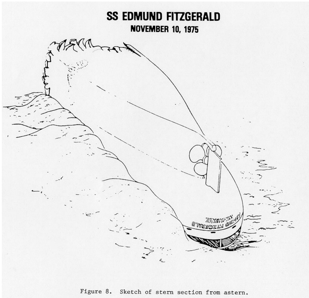
Figure 8: Sketch of stern section from astern
