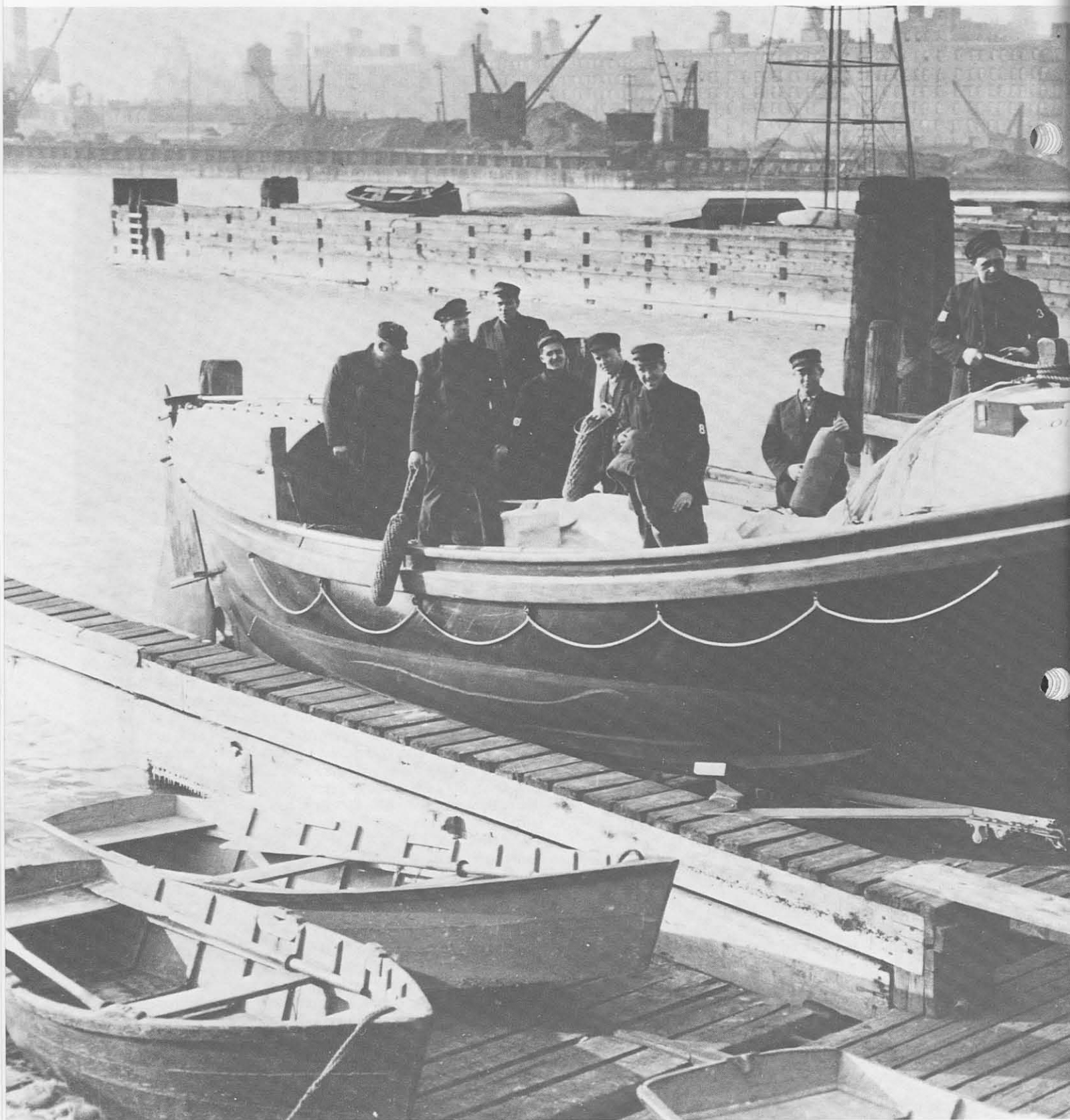
Another tool of the Life-Saving Service was the self-bailing, self-righting lifeboat. This boat was large and much heavier than the surfboat, thus not suited to all stations. Although this type boat could be launched through the surf, this in fact was not practical. Lifeboats were most commonly found at stations where marine railways could be built.
