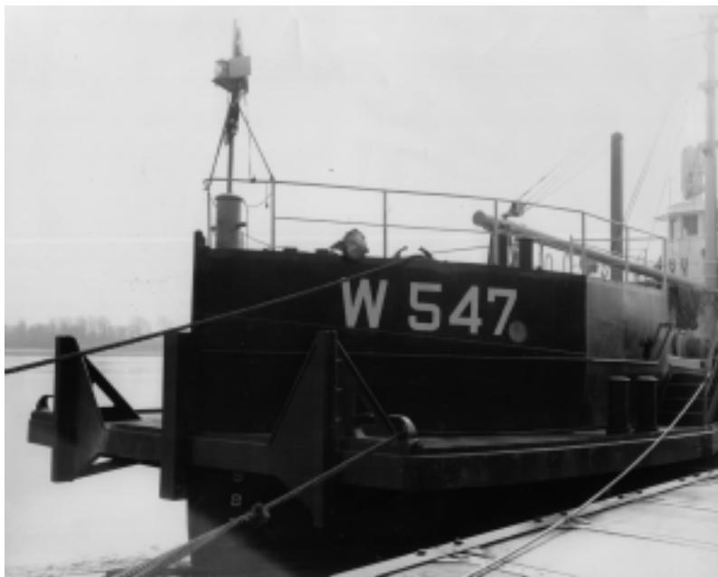
Starboard bow view showing White Pine's barge pusher. Spud, shown at right, dropped into mud to hold vessel stationary in currents (USCG photo).
