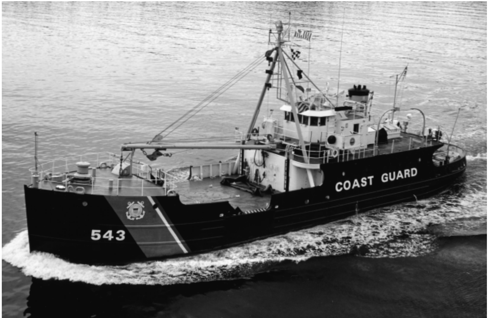
White Holly on September 10, 1968, after her single-mast and boom derrick had been replaced with a heavy-duty A-frame mast and hoisting boom system. The electric winch on deck was replaced with a hydraulic winch system housed in the superstructure behind the bulkhead (USCG photo).
