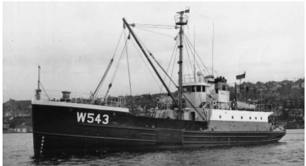
YF-339 in 1944 (National Archives photo) and White Holly (originally YF-341) in 1954 (USCG photo). Both vessels were built by the Basalt Rock Company, Inc. Coast Guard modifications included a turtle deck extending the crew berthing area from the original structure with portholes added along each side. Chain stoppers and chaffe plates were installed just aft of forecastle on maindeck, and navigation and SARS equipment added to the tower.
