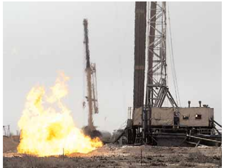
ON MARCH 12 the drilling rig operator, Chi Operating Inc., brought in blowout-control experts to cap the well. Part of the capping process involved burning off the dangerous gases, which started the next day.
