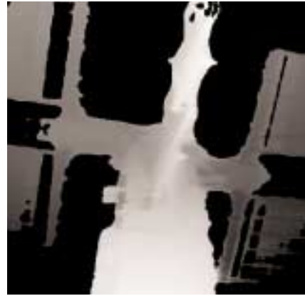
RANGE IMAGES taken with Sandia’s Laser Dynamic Range Imager, looking up the space station’s P6 mast from the Endeavour’s cargo hold, with the solar array panels extending left and right. In the left image, white represents 50 feet away and black represents 110 feet away from the camera. In the right image, each cycle from full black to full white represents 3.5 feet of range. (See “Tricks of light . . .” below.)
