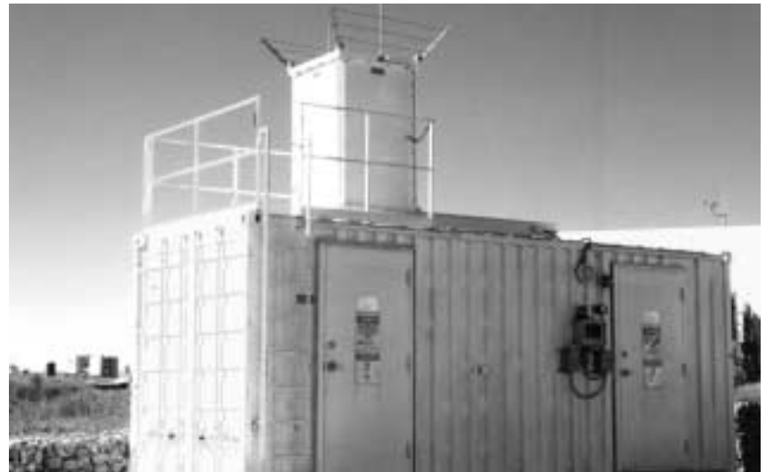
"LAB IN A BOX" — The moisture-monitoring lidar system resides in Oklahoma in a re-fitted cargo container, customized with heating, cooling, power, and an instrument table so the sensor can operate automatically around the clock.
