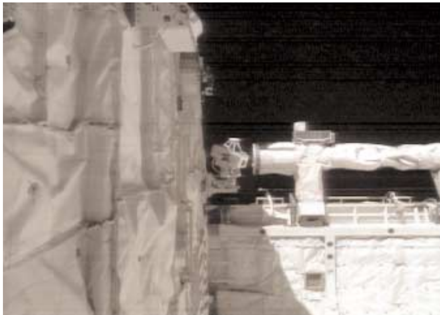
TWO VIEWS OF THE LDRI, mounted to a camera panti-tilt assembly in the port side of Endeavour’s aft payload bay (left photo, center), just left of the orbiter’s parked manipulator arm. The LDRI is the box with the small lens (top photo) mounted underneath the black-and-white camera with the larger lens.
