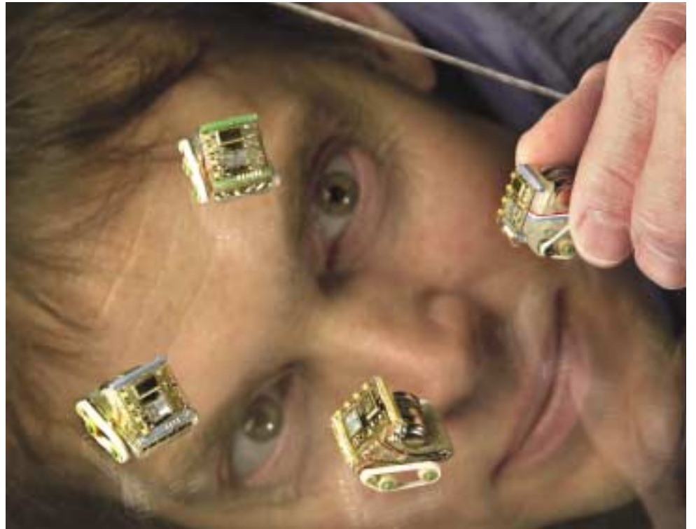
MINI-ROBOT RESEARCH — Doug Adkins (1763) takes a close-up view of the mini-robots he and Ed Heller (1763) are developing. At 1/4 cubic inch and weighing less than an ounce, they are possibly the smallest autonomous untethered robots ever created.
