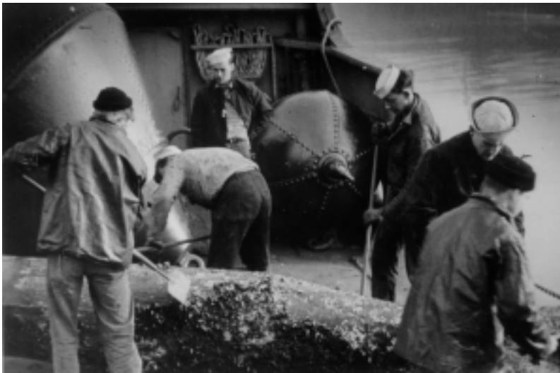
Servicing buoys aboard Fir in 1943: (Right) Bringing aboard a double bluff whistle buoy. (Below left) Scraping off sea growth. (Below right) Preparing scraped and repainted buoys for relief. Photos courtesy National Archives, Seattle.
