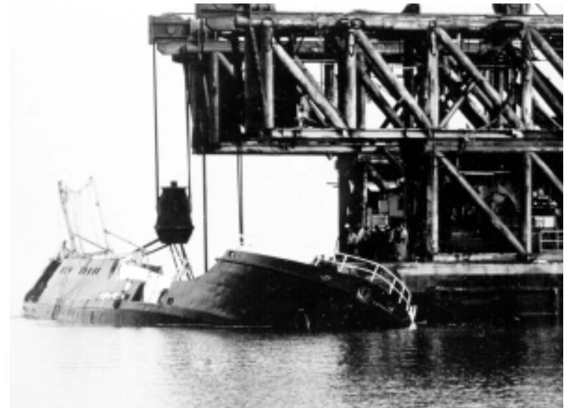
Mesquite's hull is lowered to its final resting place in Lake Superior. The tender ran aground on rocks several months earlier and was battered by winter storms. The wrecked vessel became part of an underwater preserve and is regularly visited by recreational divers.
