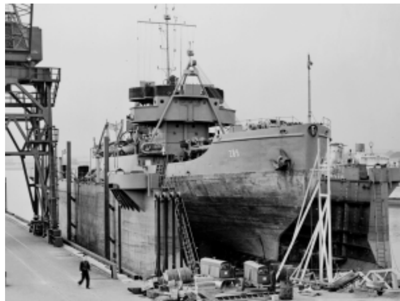
Woodbine in drydock at the U.S. Coast Guard shipyard. This views shows the notched or cutaway forefoot that made the 180s suitable for icebreaking.
