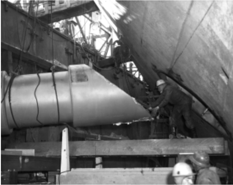
Cowslip rests in a drydock as shipyard workers install a bowthruster. The addition of bowthrusters made the single-screw buoy tenders more maneuverable.
