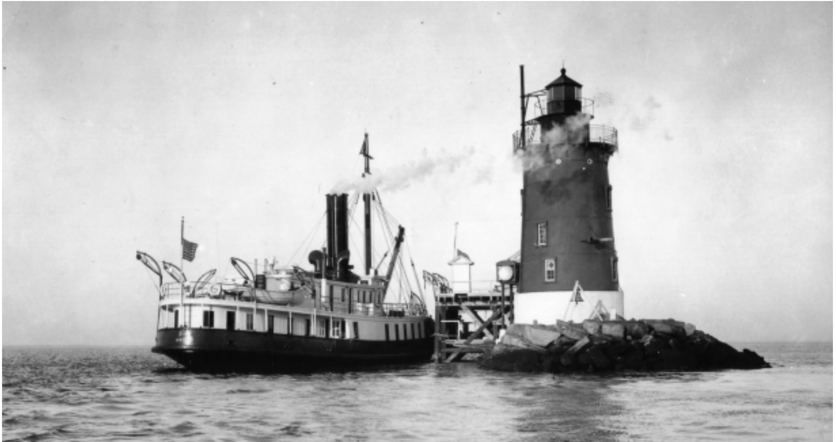
Early buoy tenders were called lighthouse tenders. Here USLHT Iris services a lighthouse. Commissioned in 1899, this was the second tender to be named 'Iris'. A 180-foot U.S. Coast Guard cutter was also given that name.
