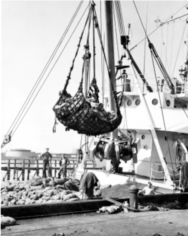
An "A" class buoy tender loads cargo alongside a dock. The cargo-carrying capacity of the 180s made them useful in supplying out-of-the-way settlements and installations. Note the A-frame support for the cargo boom. This system was found only on "A" class tenders.
