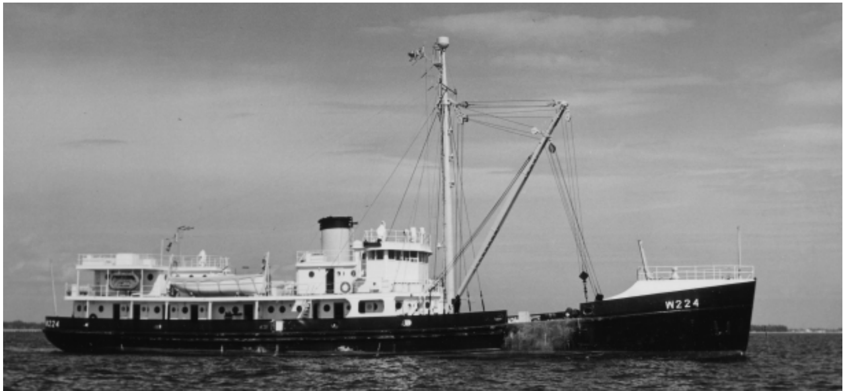
The design of the 180s was adapted from that of the 177-foot Juniper constructed in 1939. Alterations were made based on the requirements of the newly-expanded Coast Guard. Juniper is shown here underway in 1949.
