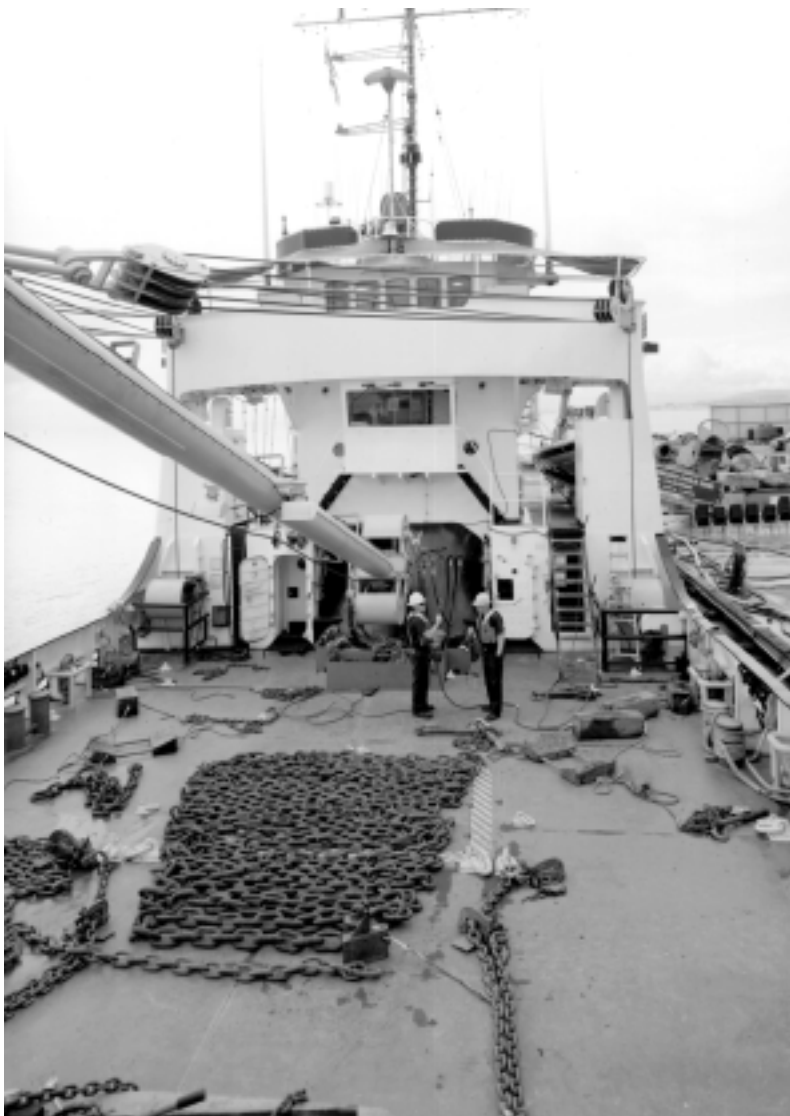
Buttonwood's buoy deck with mooring chains laid out. HABS/HAER photo by Jet Lowe.
