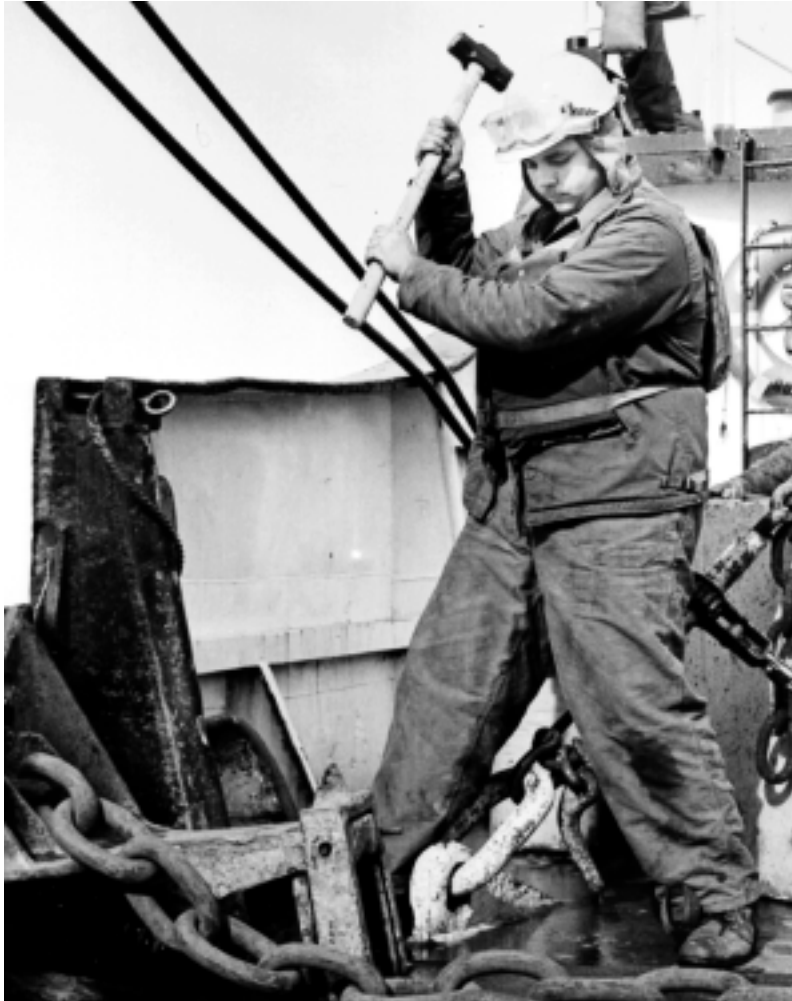
A member of a buoy tender's deck force prepares to trip the chain stopper. This will release the buoy's anchor for the plunge to the sea-floor.
