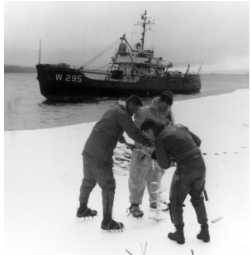
Officers from Evergreen drill a hole in an iceberg. They later placed explosives in the hole and detonated the charge as part of experiments to determine the effect explosives would have on icebergs.
