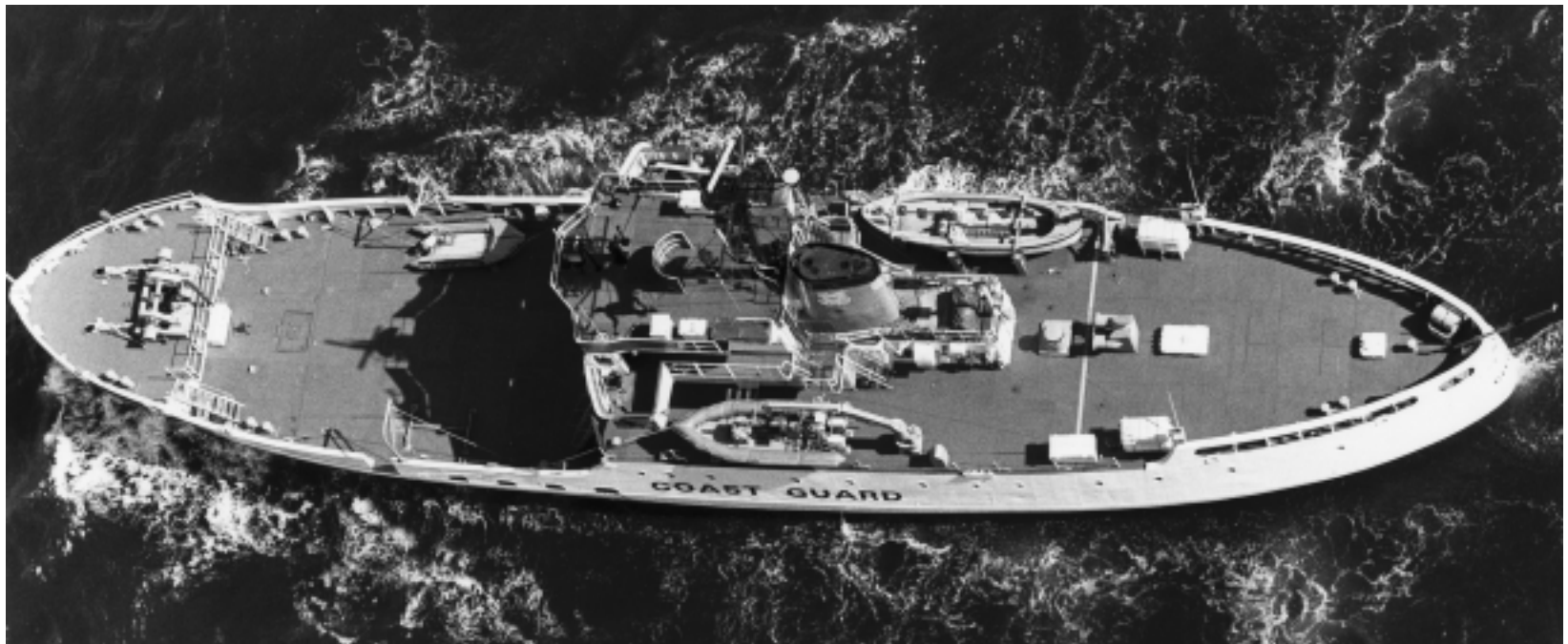
Aerial view of Citrus underway. This photo was taken after her conversion to a medium-endurance cutter. Note the white hull and absence of buoy handling equipment.
