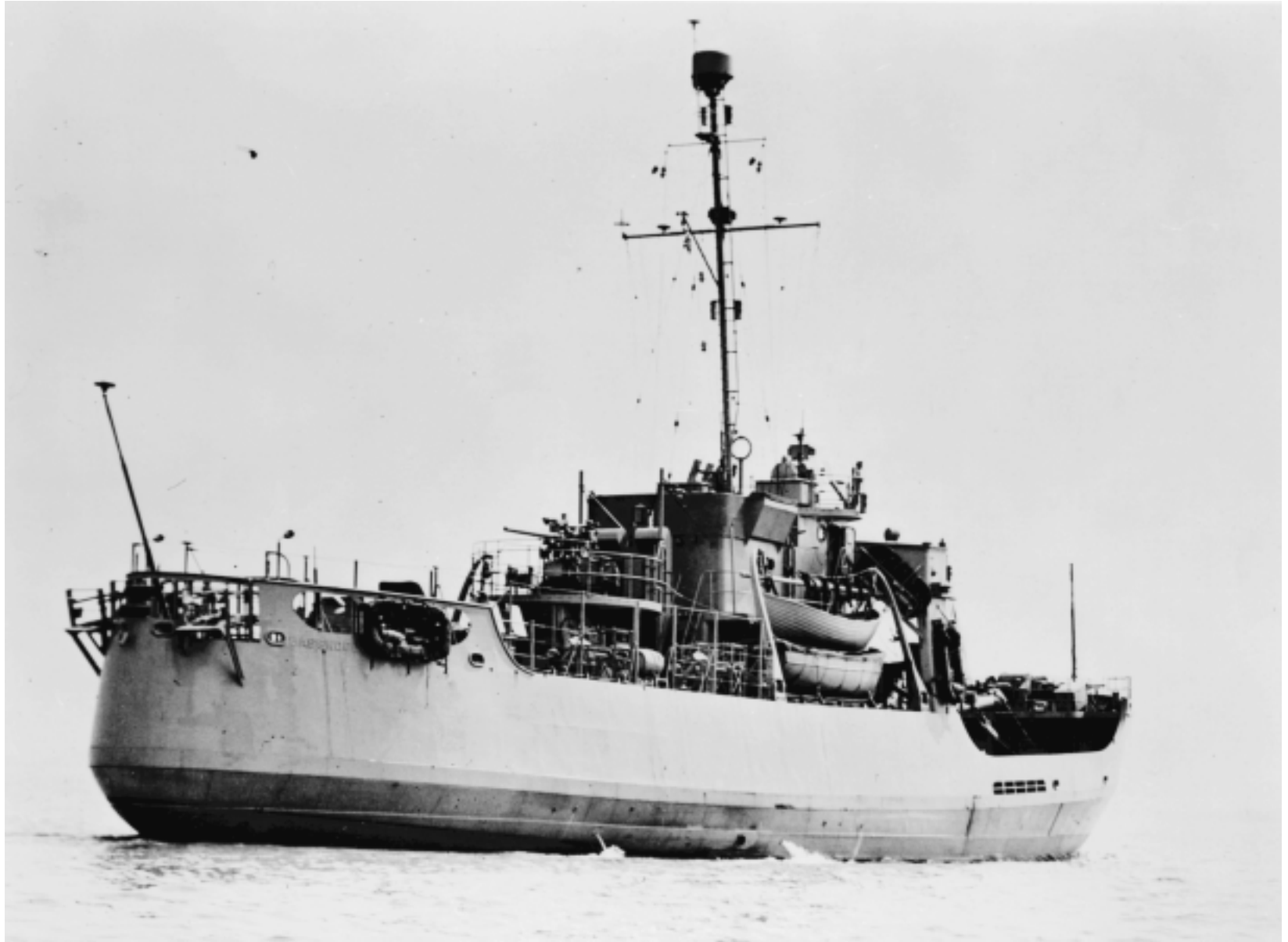
Basswood underway during World War II. Depth charge launchers are clearly visible in the stern section.
