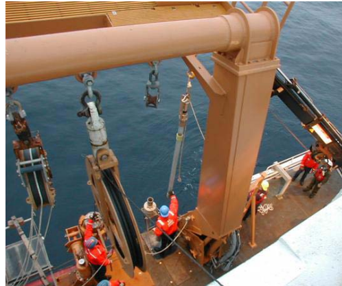
Connecting the trigger core to the JPC for deployment
