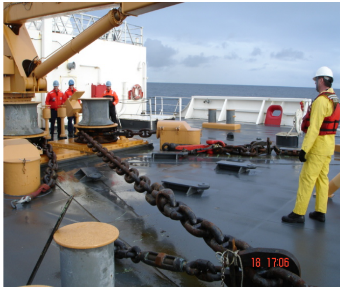
Anchor solution showing the port anchor chain connected to the starboard anchor
