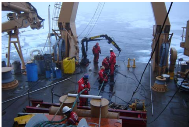
Deploying the seismic air guns and acoustic streamer
