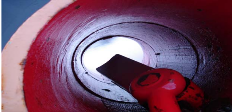
The remaining anchor shank after loss of the port anchor
