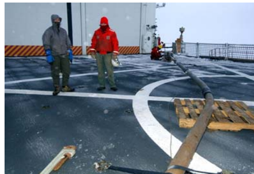
Badly bent JPC recovered on the flight deck
