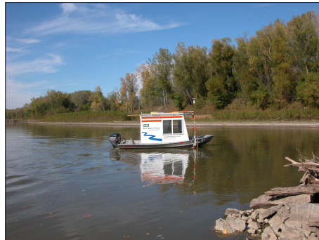
CERC scientists use hydroacoustic mapping and hydraulic modeling to assess sturgeon habitat dynamics and availability in the Missouri River.
