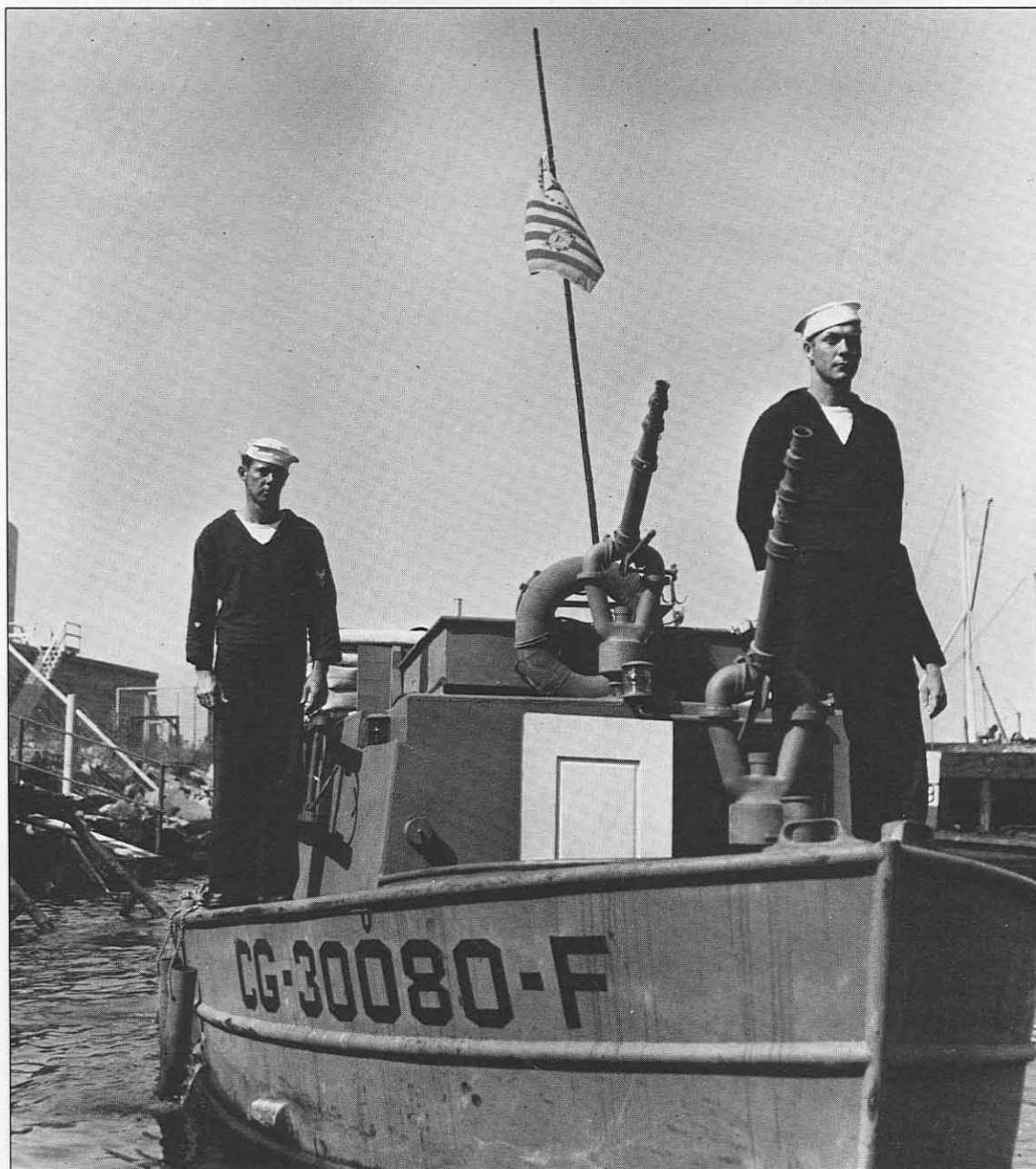
Left: The 30-foot Hanley fireboats, built in 1942-1943, had four 500-gallon-a-minute fire pumps.
