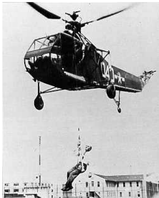
Figure 5. HNS-1 with hoist. Note. From Rotary Action. Notes on history of helicopters. Retrieved April 2, 2008, from http://rotaryaction.com/history.html .
